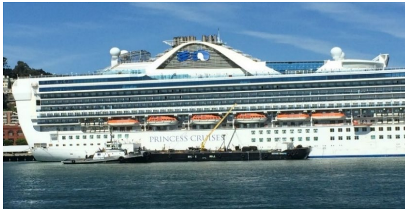
Figure I-3. Bernie Briere Double Hull Fuel Bunker Barge at Port of San Francisco
