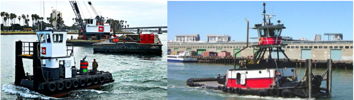
Figure I-20a and Figure I-20b. Near Shore Pushing Vessels
