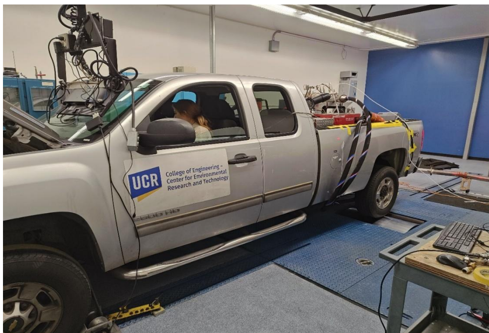
Figure 44. The fully instrumented test vehicle operating on a chassis dynamometer during the second phase of pilot testing.
