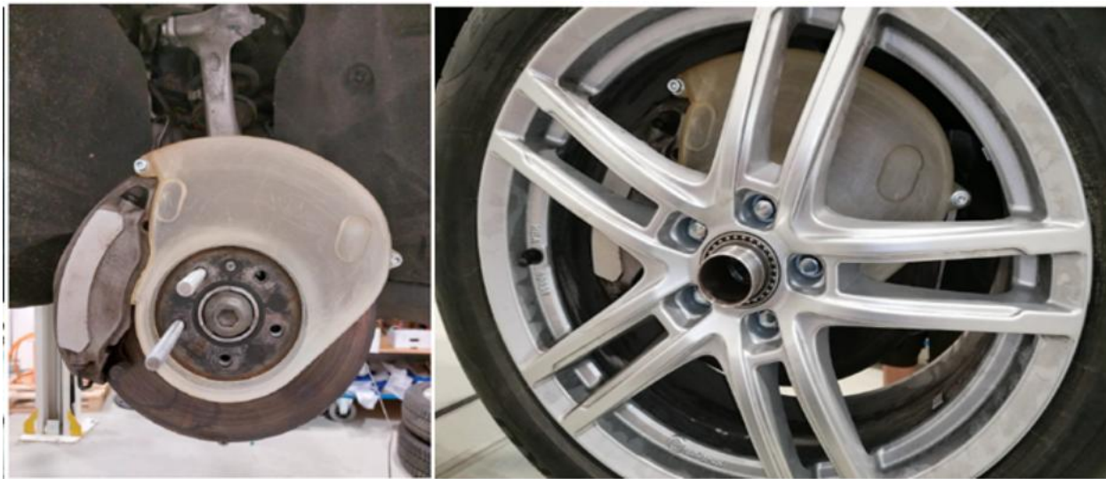
Figure 10. The AVL partial enclosure method with center hub outlet.
