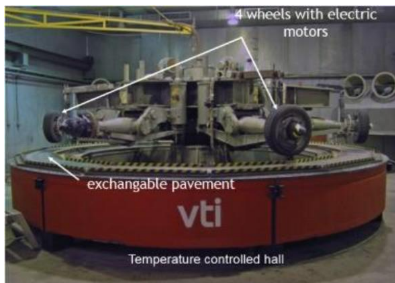
Figure 4. The VTI turntable-style roadway simulator (Grigoratos et. al., 2018).
