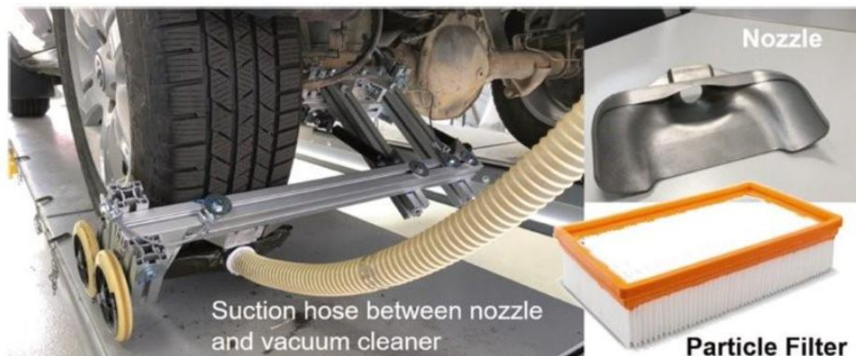
Figure 17. The sampling setup used by Continental Tire, in which a tire doped with TiO 2 was used as a marker to determine the tire-sourced percentage of collected TRWP.
