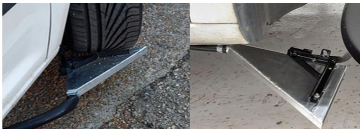
Figure 13. The Ricardo-developed tire sampling system utilized for characterization of PM emitted from the tire/road interface.
