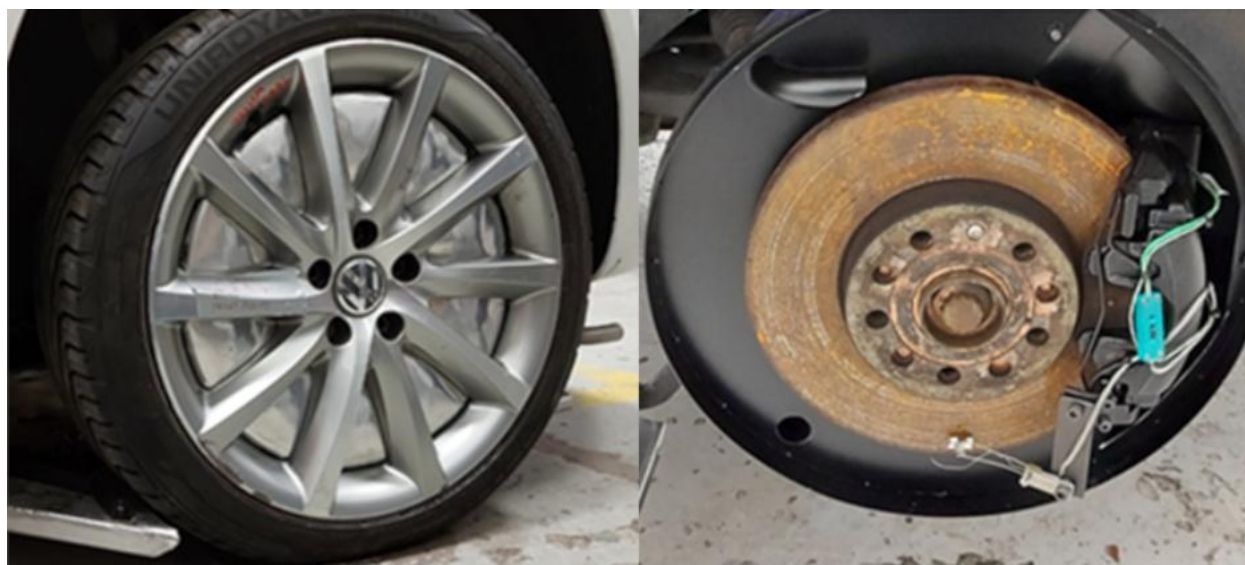
Figure 6. The Ricardo light-duty full enclosure brake PM sampling system.
