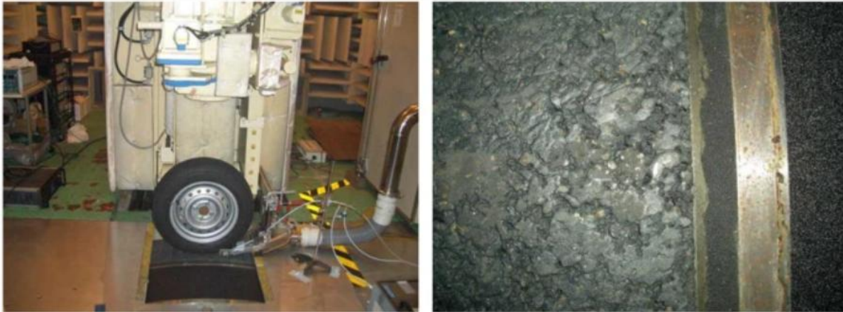
Figure 2. The external rotating drum tire test rig at JARI (left) with a closeup of the epoxied roadway simulation media (right).
