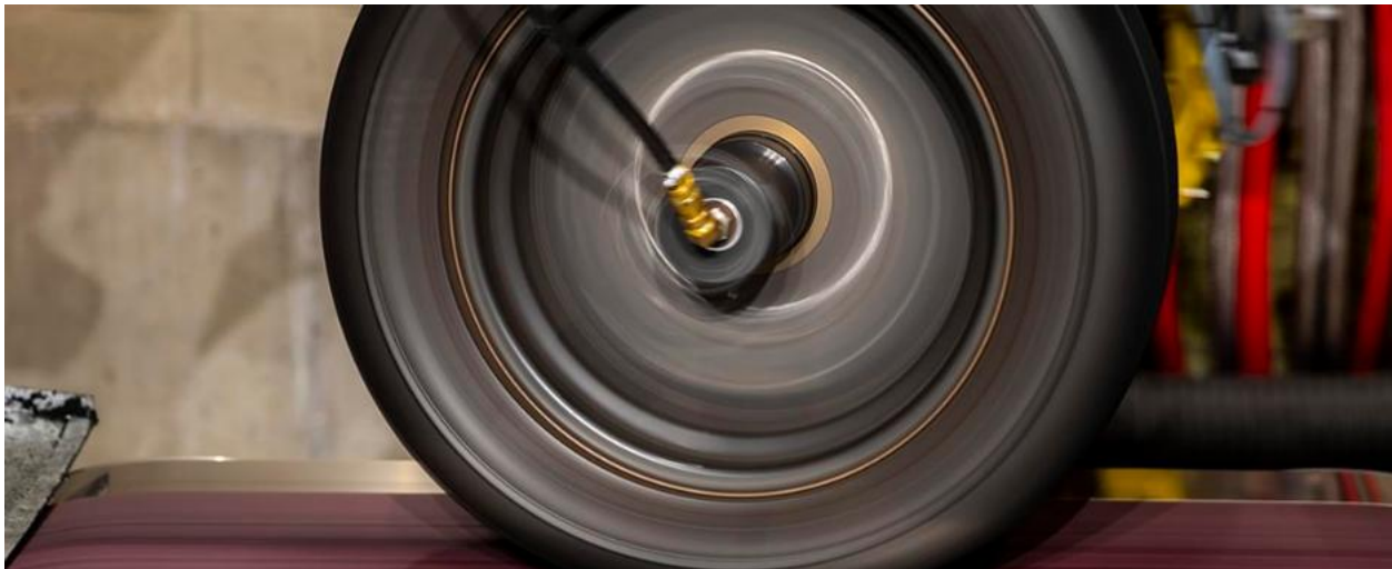
Figure 5. The Smithers force and moment test rig.
