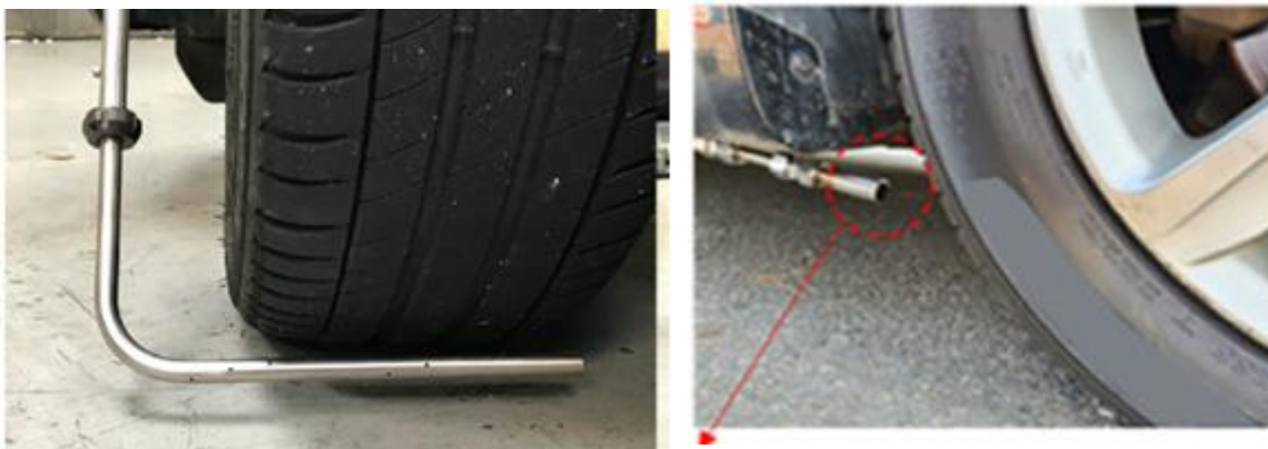
Figure 14. Sample probes used in tire/road interface PM sampling for the intention of studying particle characteristics but not estimating mass emission factors.
