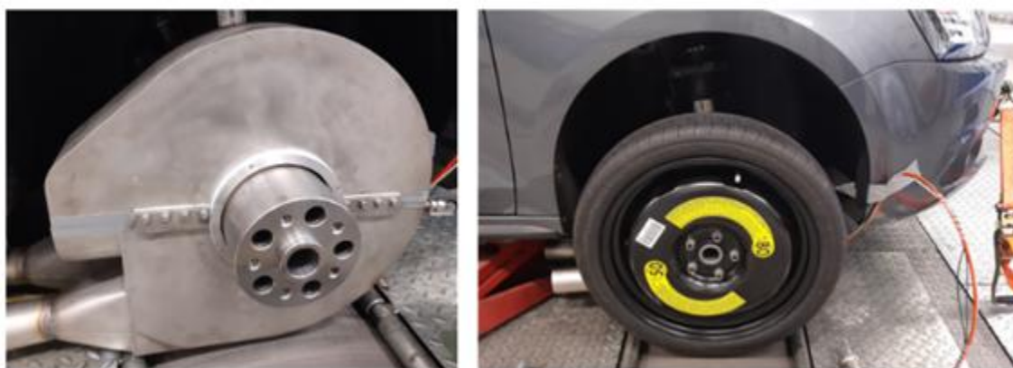
Figure 8. The brake PM enclosure developed by the Swiss Federal Laboratories.
