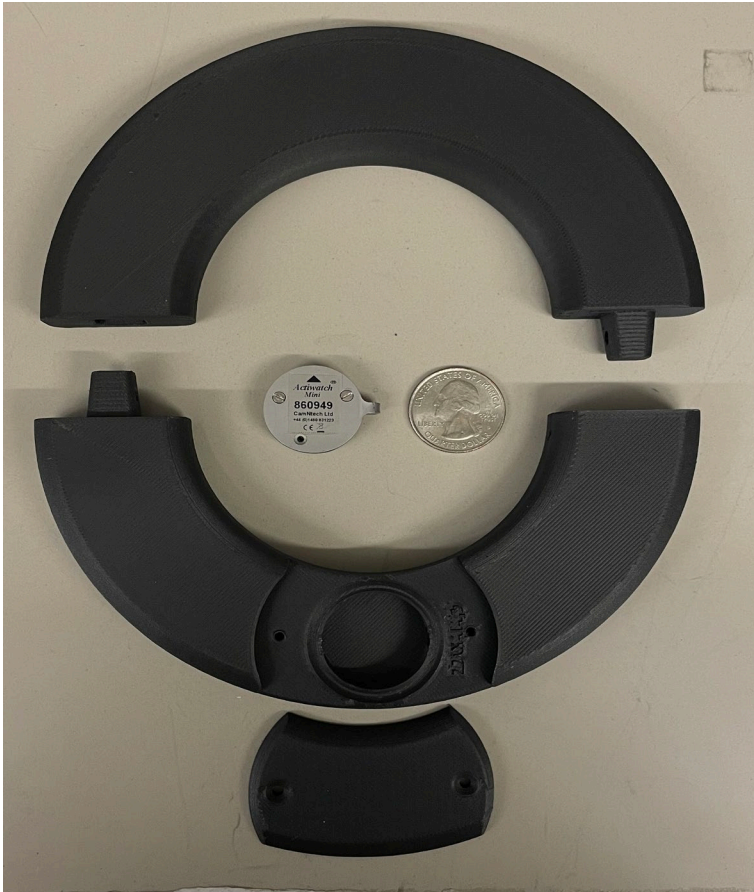
Figure 15. 3D-printed nylon collar with Actiwatch mini (quarter for scale).
