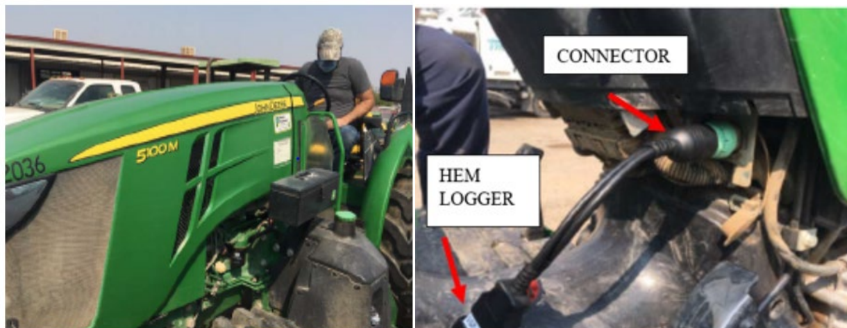
Figure 2-4. Installation of HEM Data Logger on a Typical Farm Tractor
