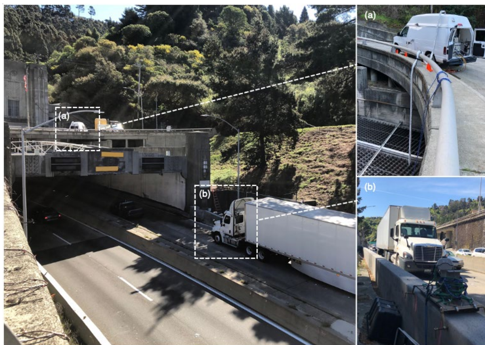
Figure 1. Instrumented van positioned on an overpass at the Caltrans facility at the Caldecott Tunnel, sampling the exhaust from a truck as it travels eastbound on Highway 24 and enters Bore 1 of the tunnel. The van is circled in the wide-view image and shown in more detail in the inset picture (a), and the roadside camera positioned at the entrance to the tunnel is also circled and shown in (b). Reproduced from Preble et al. 7
