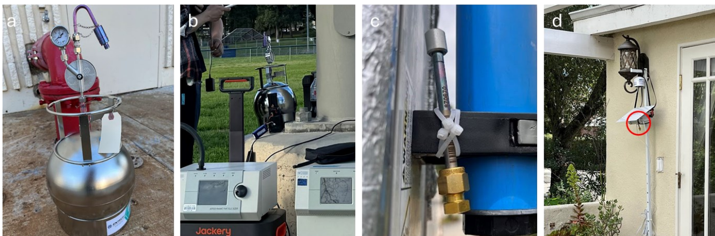
Figure 2. Photos of the proposed sampling devices. (a) The Summa canister, (b) the Summa canister sampling in the field, (c) the diffusion tube, and (d) the diffusion tube sampling in adjacent outdoor residential areas, with the red circle indicating the diffusion tube.
