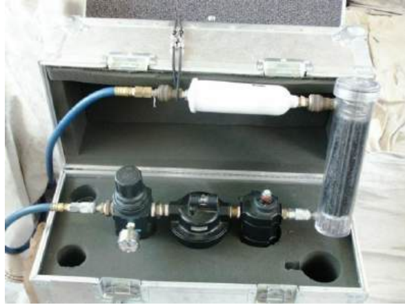
Figure A-3 Field Processing Unit for Purifying Dilution Air in Carrying Case
