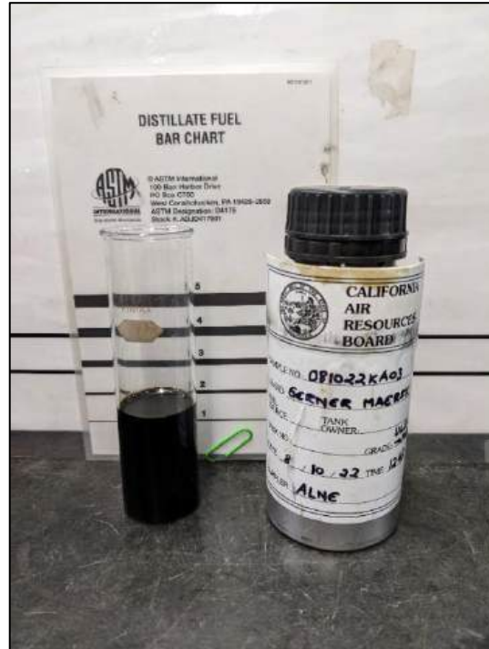
Figure 7. 081022KA03 taken at 1245 hours, represents the sample of MGO just approaching the time of sulfur compliance
