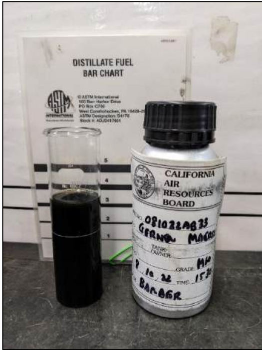
Figure 8. 081022AB33 taken at 1530 hours, represents the sample of MGO just approaching the time of Carbon Residue compliance
