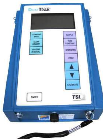
Figure A-5 Picture of TSI DustTrak
