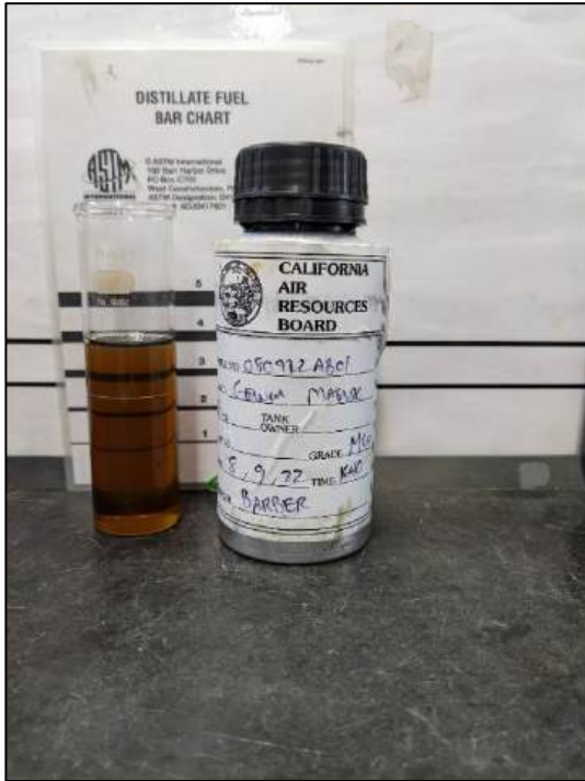
Figure 6. 080922AB01 represents the clean sample of uncontaminated MGO at the beginning of the
