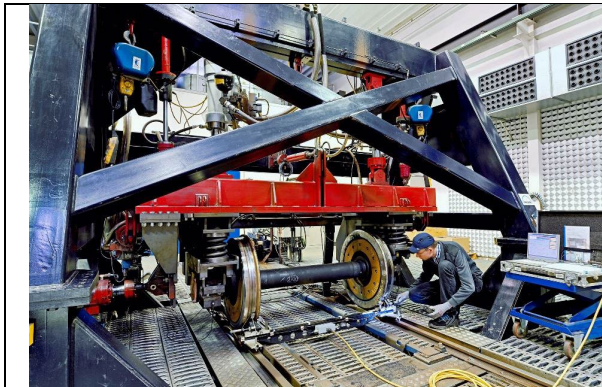
DB Test rig A during normal low- and high-speed wear and tribology testing using a full axle-set with two wheels under loading to reflect the test cycle
