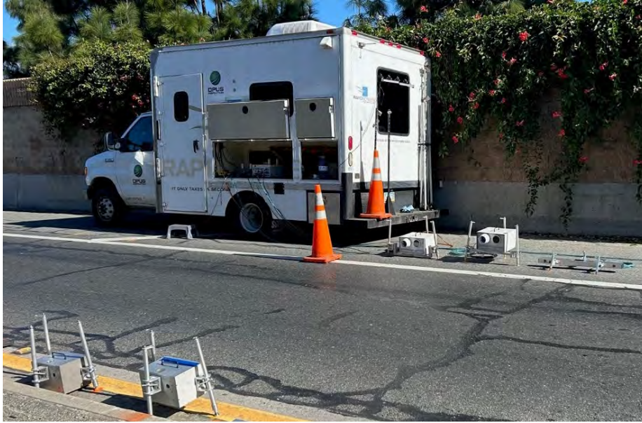
Figure 2. An Opus roadside RSD unit set up on a highway onramp.
