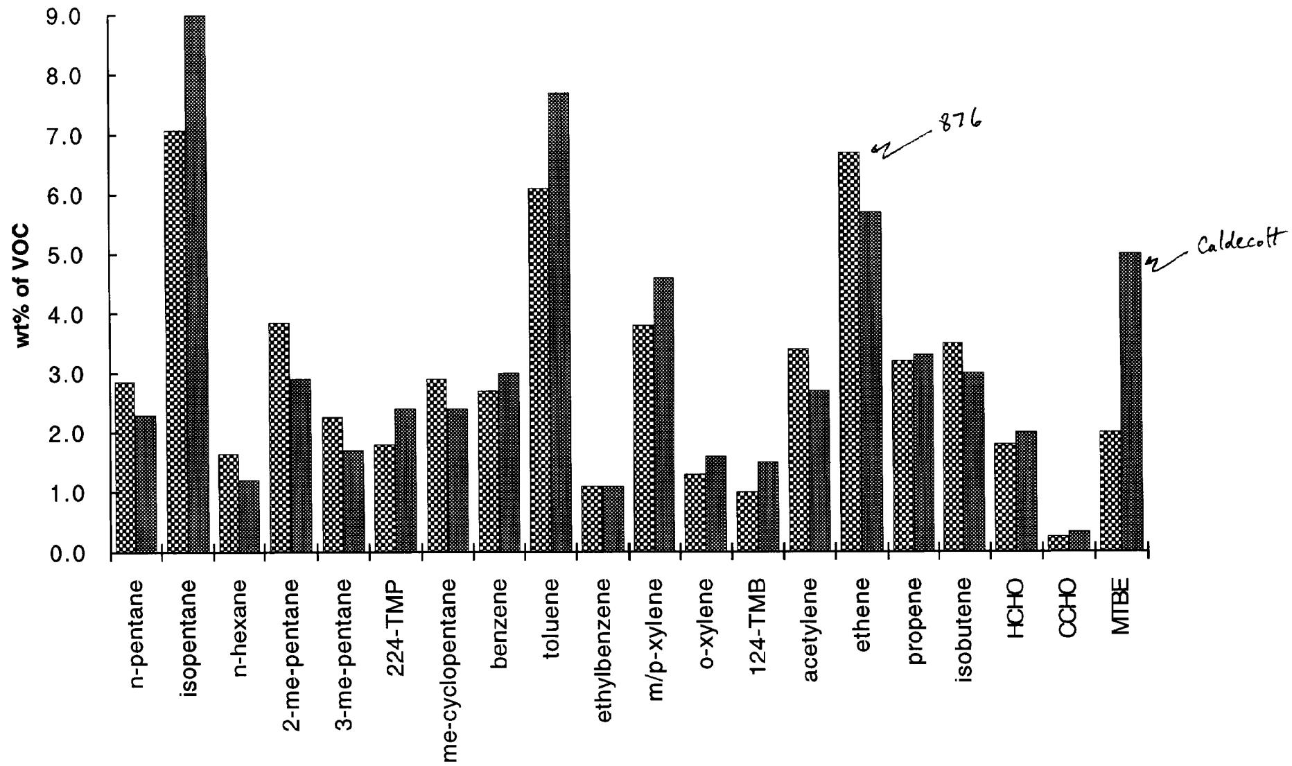
Figure 2: Comparison of Stabilized Exhaust Profiles for RFG with MTBE (876), 2% as ETOH (663), 3.5% as ETOH (673), and w/o oxy (653), in that order
