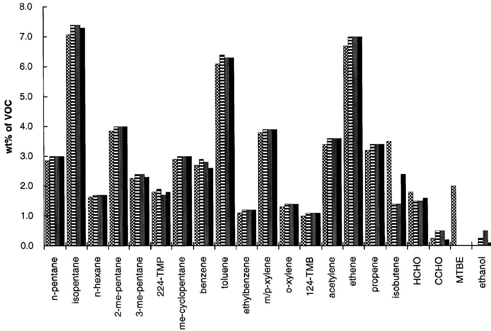
Figure 3: Comparison of Exhaust Speciation Profiles for RFG with MTBE (Profiles are CAT STAB, CAT STRT, NON-CAT STAB, and NON-CAT STRT in that order)
