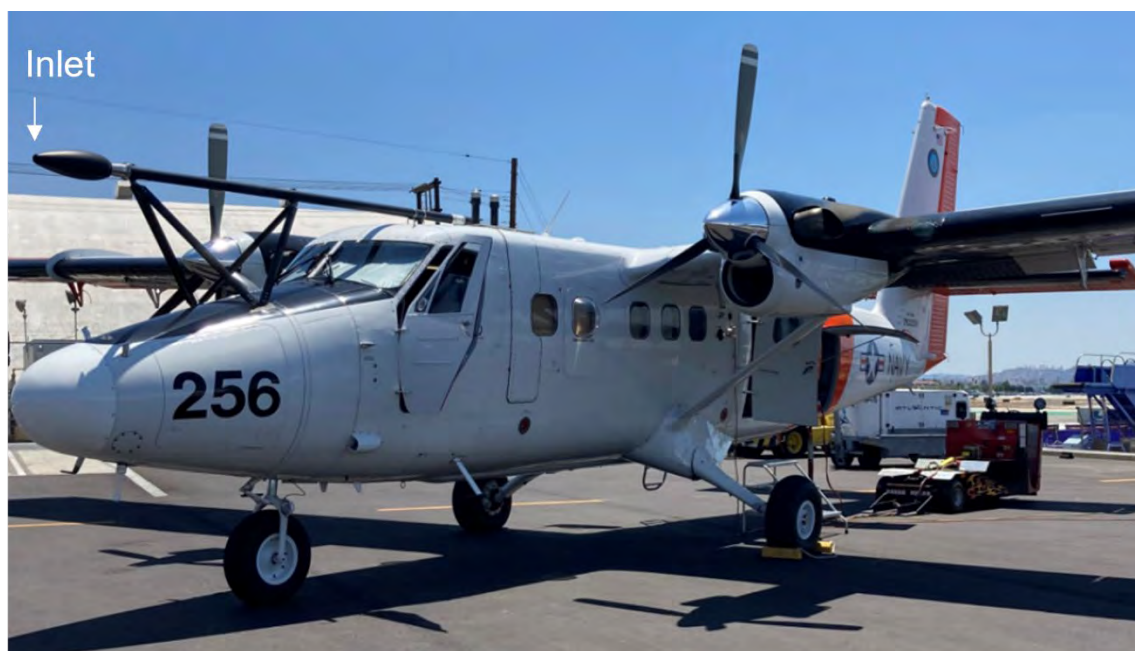
Fig. 2.3. Twin Otter aircraft with mounted inlet.
