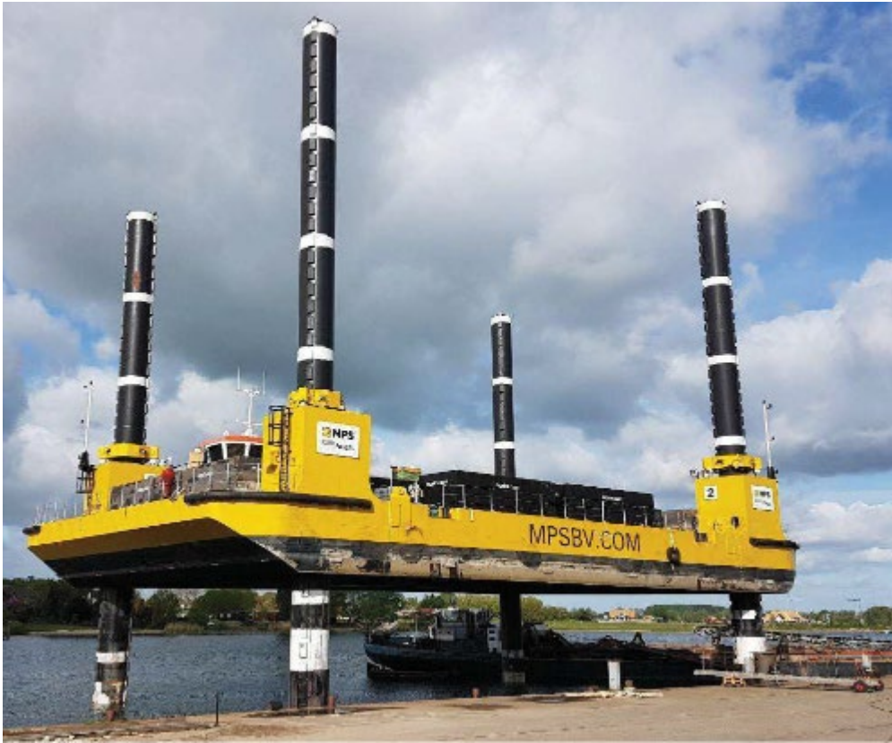
Figure 7-3 Jack-up barge example
