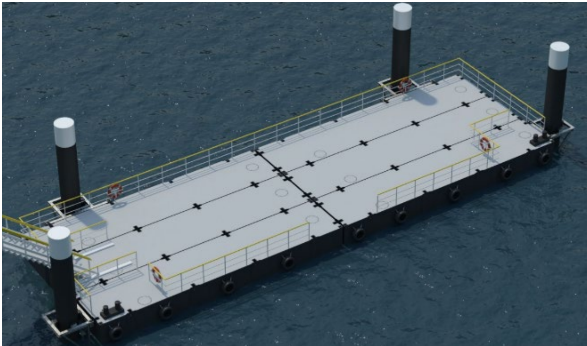
Figure 7-2 Spud barge example
