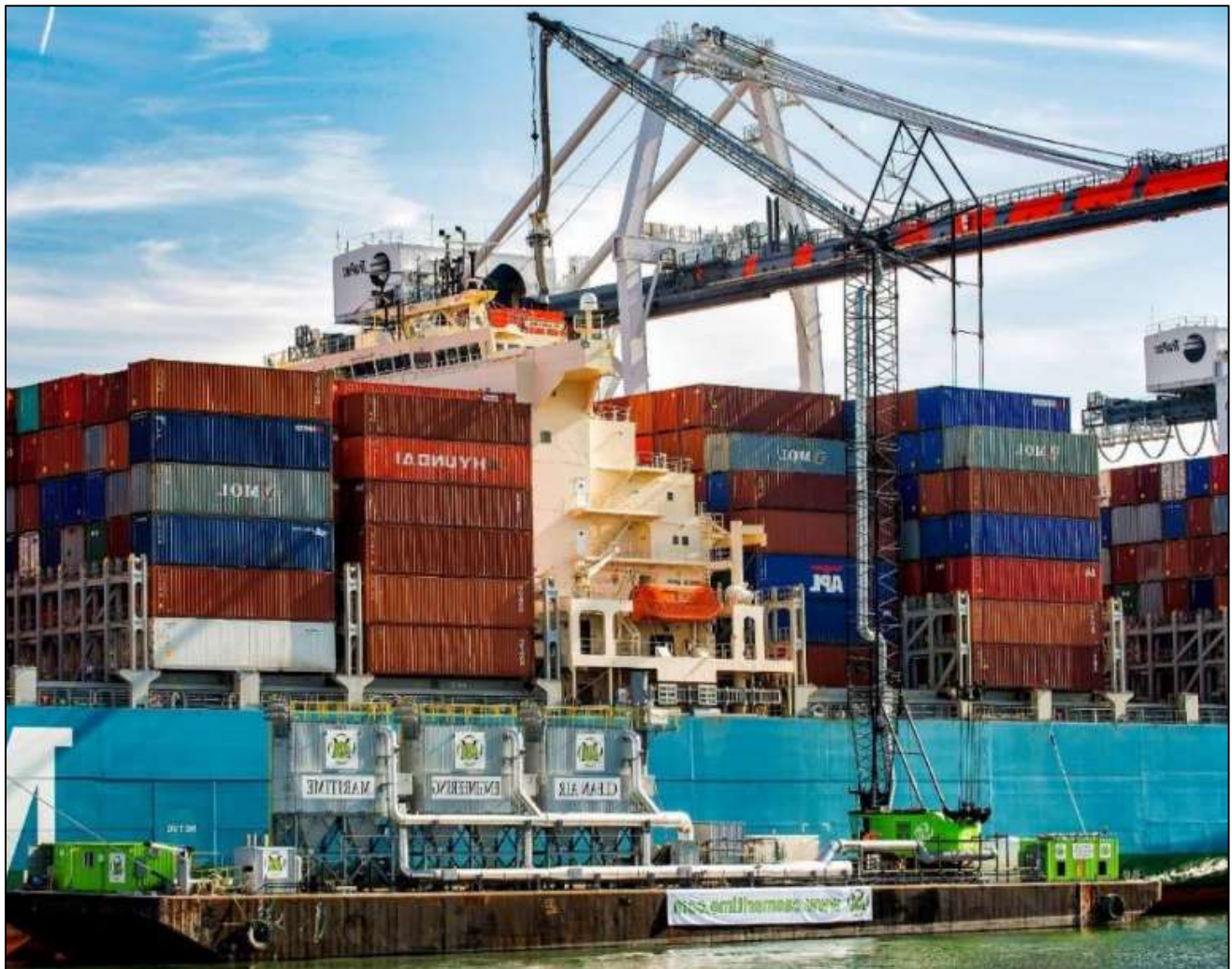
Figure 10: Barge-Based Capture and Control System for Container Vessels (CAEM)
