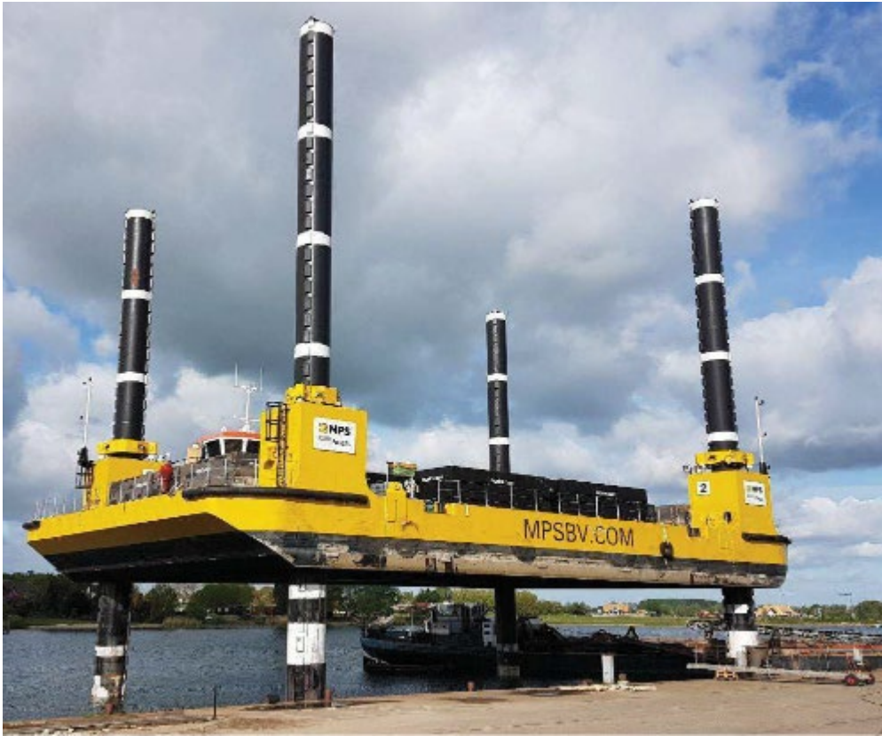
Figure 7-3 Jack-up barge example
