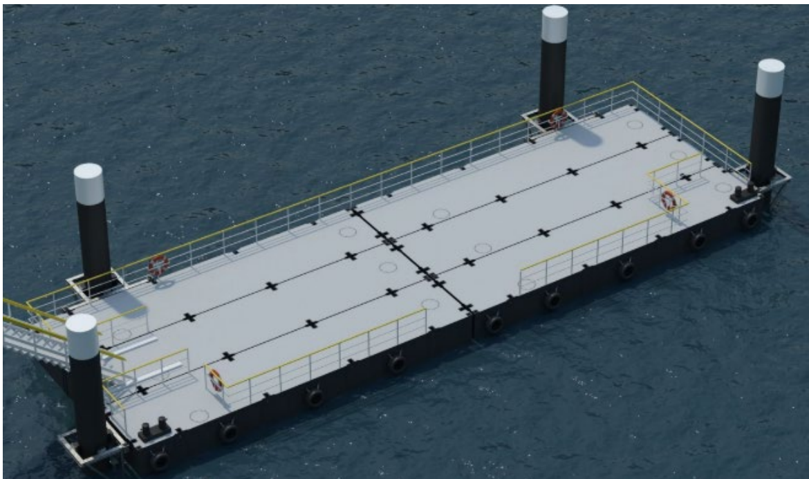
Figure 7-2 Spud barge example
