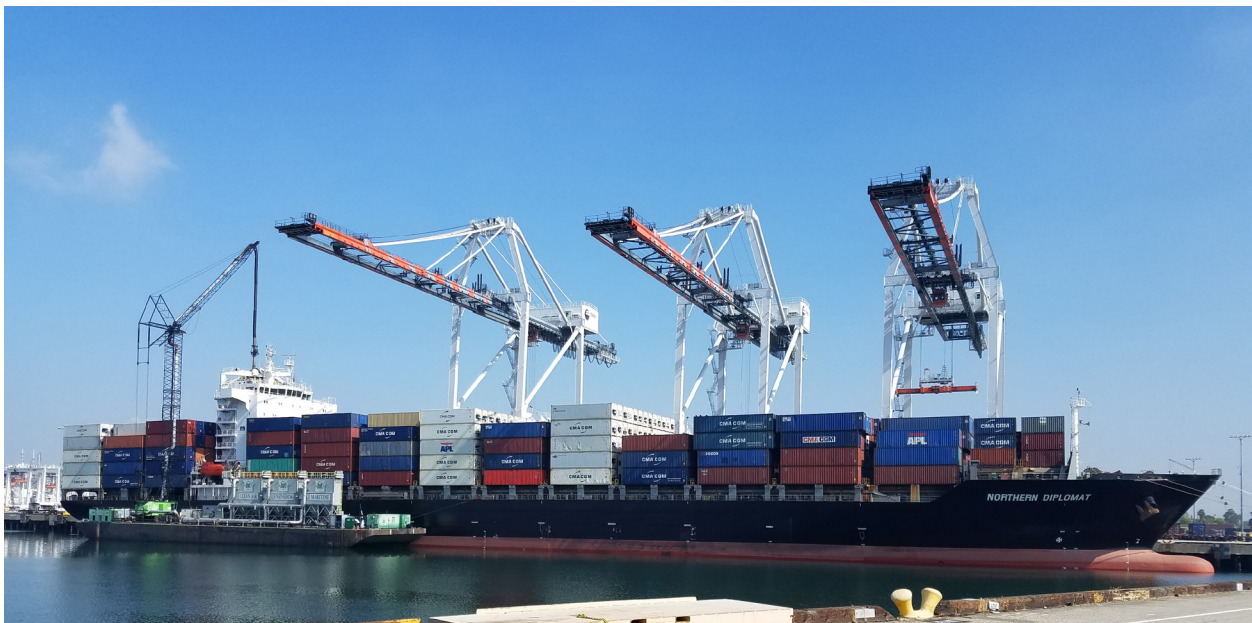
FIGURE 9: A CAPTURE AND CONTROL SYSTEM CONTROLLING EMISSIONS ON A CONTAINER VESSEL
