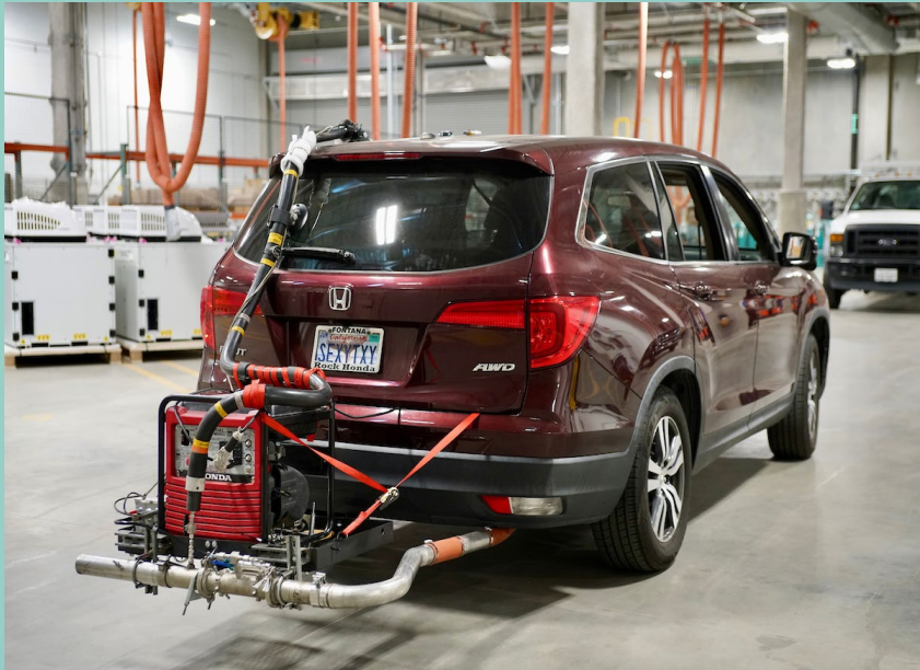
Light-Duty Vehicle Surveillance Program Dynamometer (Dyno) and Portable Emissions Measurement Systems (PEMS)
