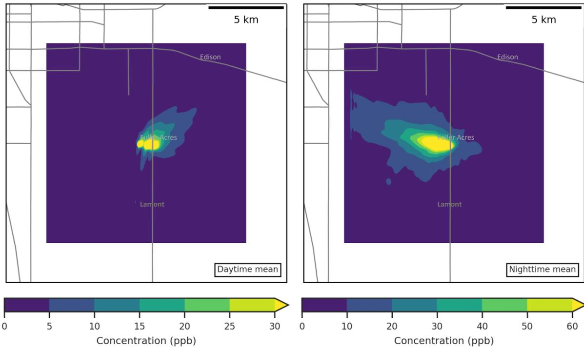
Figure 102 Mean daytime (left panel) and nighttime (right panel) concentrations in the plume dispersion simulations for Kern Oil refinery during the periods October 12-14 and October 19-21.
