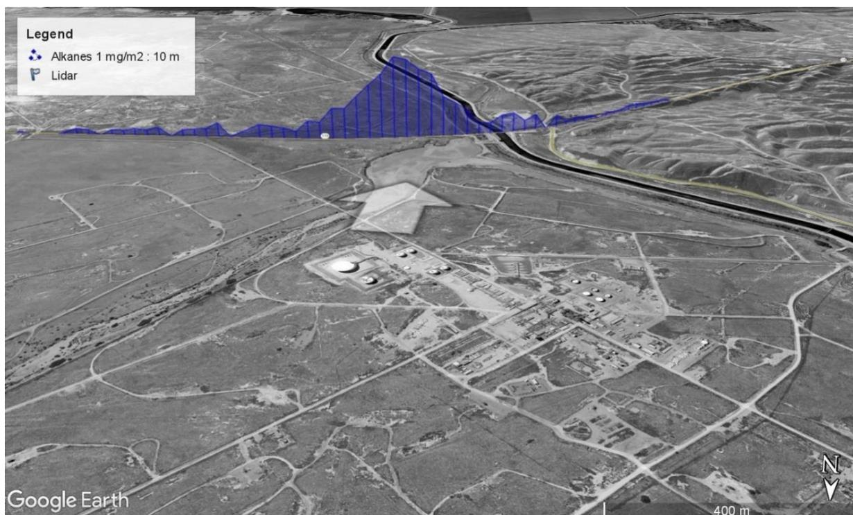
Figure 32. Alkane emission measurement of the Coles Levee North field on 14 October 2021 , 11:40. Wind was blowing from north as indicated by the enclosed white arrow. The blue curve marks measured alkane column, where the height is scaled with the column having 1 mg/m<sup>2</sup> correspond to 10 m height above ground. Map from Google Earth™, 2021.
