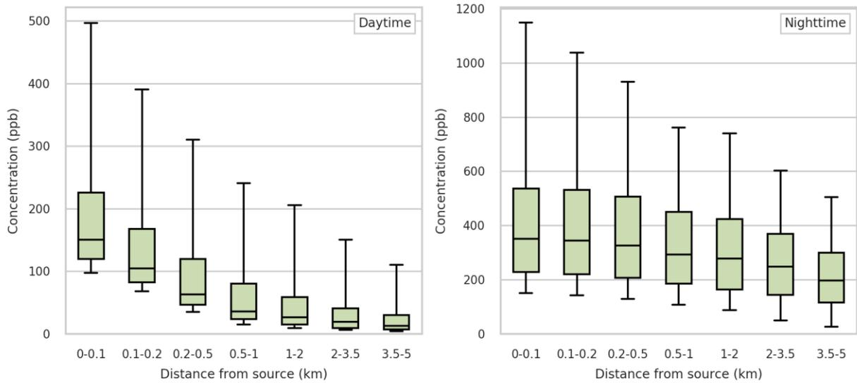
Figure 104 Box plots illustrating the distributions of plume max concentrations for different distance intervals from the source in the simulations for the Kern Oil refinery . The boxes indicate lower quartiles, medians, and upper quartiles, while the whiskers indicate 5<sup>th</sup> and 95<sup>th</sup> percentiles. The left panel shows daytime distributions, while the right panel shows night-time distributions.
