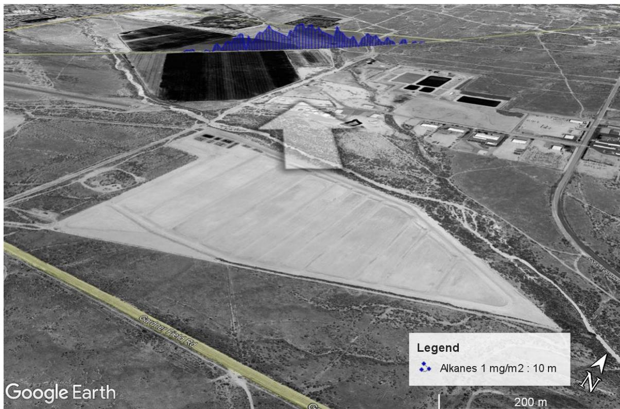
Figure 45. Alkane emission measurement from the Taft pond on 16 October 2019, 12:50. The height of the blue contour corresponds to the measured column of alkanes where 10 m equals 1 mg/m<sup>2</sup>. The white arrow indicates the average wind direction during the measurement. Map from Google Earth™, 2021.
