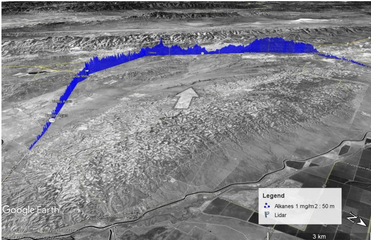
Figure 31. Alkane emission measurement of the Elk Hills field on 17 October 2021, 14:10. Wind was blowing from north-east as indicated by the enclosed white arrow. The blue curve marks measured alkane column, where the height is scaled with the column having 1 mg/m<sup>2</sup> correspond to 50 m height above ground. Map from Google Earth™, 2021.
