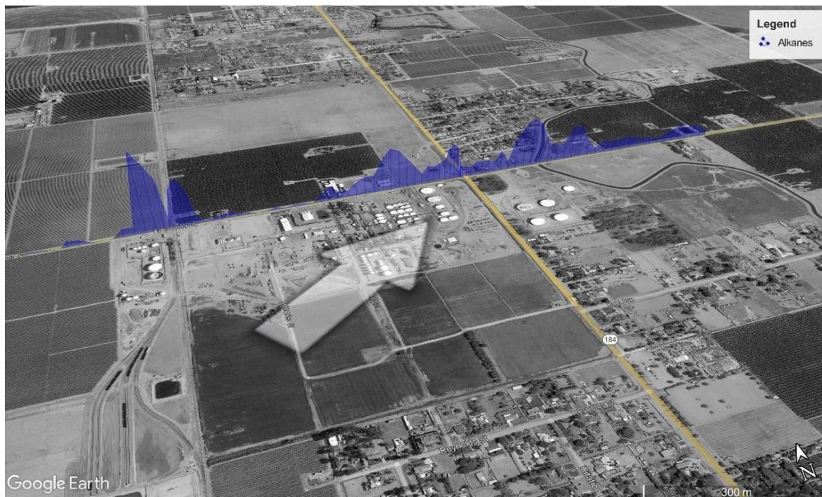
Figure 38. Typical SOF Alkanes measurement of the Kern Oil Refinery. The height of the blue contour corresponds to the measured column of alkanes where 10 m equals 1 mg/m<sup>2</sup>. The white arrow indicates the average wind direction during the measurement. Map from Google Earth™, 2021.
