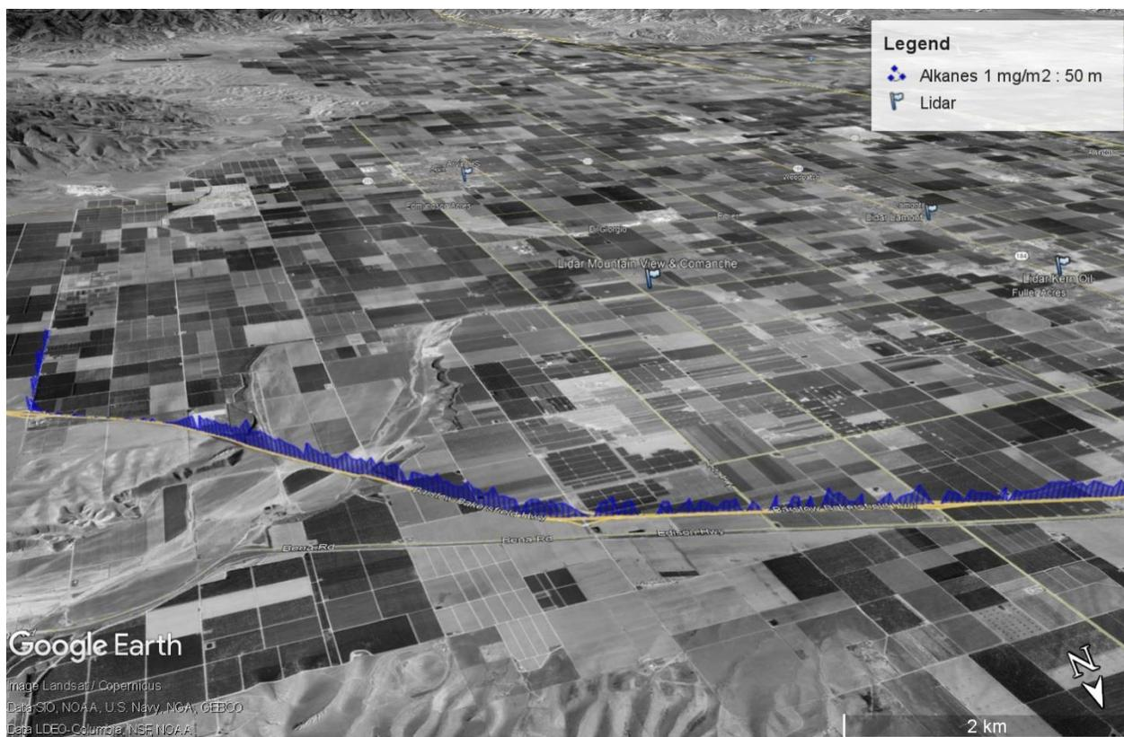
Figure 35. Alkane emission measurement by SOF of the Edison and Mountain View oil fields 13 October 2021, 11:50. The height of the blue contour corresponds to the measured column of alkanes where 50 m equals 1 mg/m<sup>2</sup>. The white arrow indicates the average wind direction during the measurement (e.g. south-westerly wind here). Map from Google Earth™, 2021.
