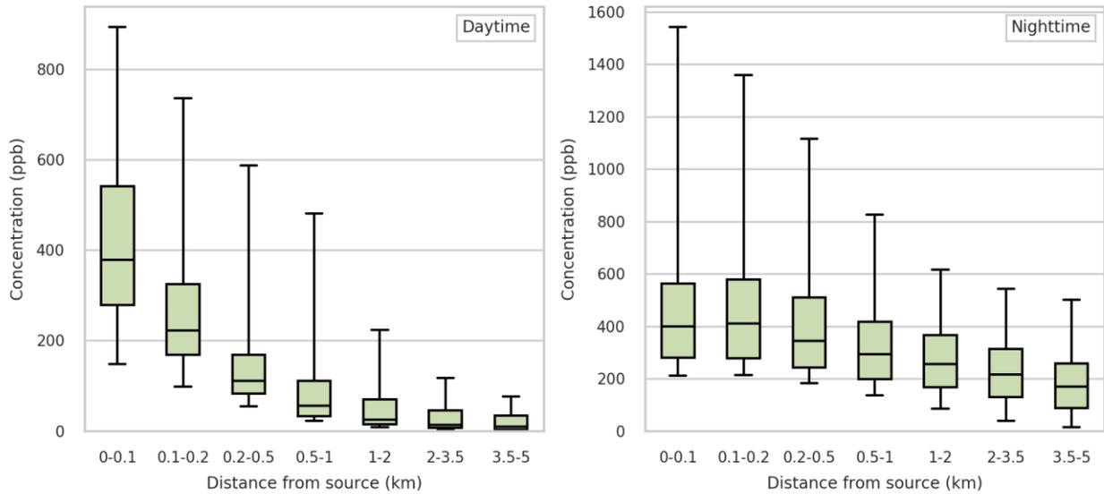
Figure 109 Box plots illustrating the distributions of plume max concentrations for different distance intervals from the source in the simulations for Lost Hills Processing 1. The boxes indicate lower quartiles, medians, and upper quartiles, while the whiskers indicate 5<sup>th</sup> and 95<sup>th</sup> percentiles. The left panel shows daytime distributions, while the right panel shows night-time distributions.
