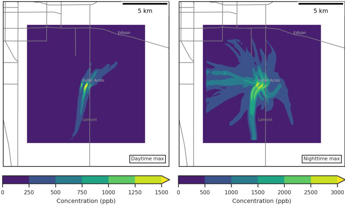
Figure 101 Maximum daytime (left panel) and nighttime (right panel) concentrations in the plume dispersion simulations for Kern Oil refinery during the periods October 12-14 and October 19-21.
