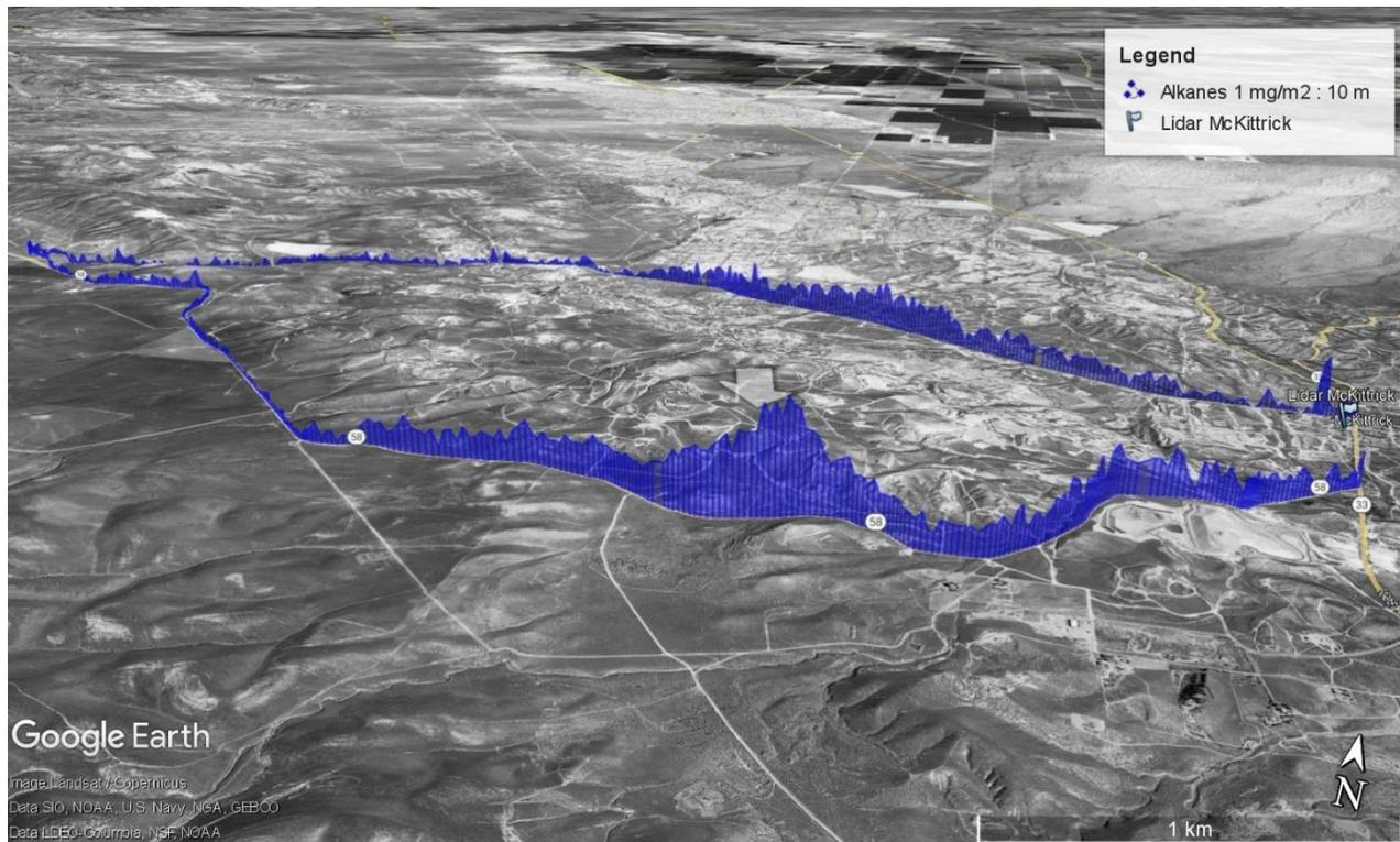
Figure 29. Alkane emission measurement of the McKittrick field on 29 September 2021 , 14:05, with the Cymric field upwind. Wind was blowing from north-northwest as indicated by the enclosed white arrow. The blue curve marks measured alkane column, where the height is scaled with the column having 1 mg/m<sup>2</sup> correspond to 10 m height above ground. Map from Google Earth™, 2021.
