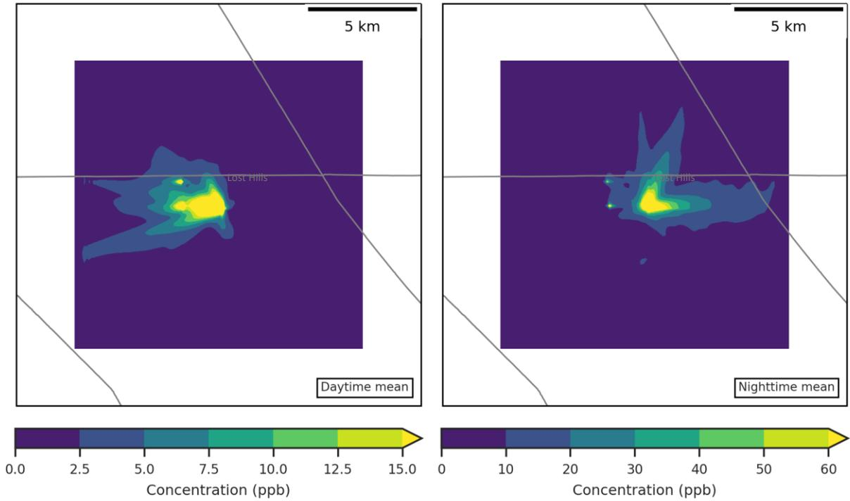
Figure 107 Mean daytime (left panel) and nighttime (right panel) concentrations in the plume dispersion simulations for Lost Hills Processing 1 during the period 17-22 October 2021.
