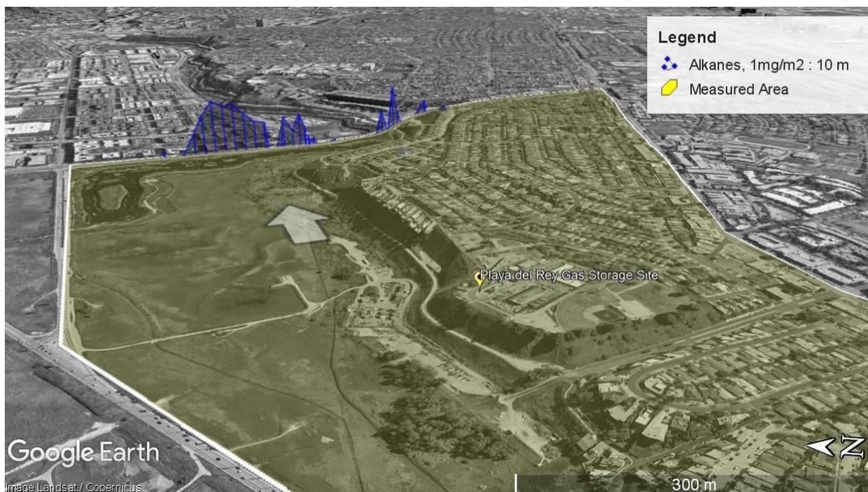
Figure 43 SOF Alkane measurement of Playa Del Rey Gas Storage Site 25 June 2021 at 11:36. The height of the blue contour corresponds to the measured column of alkanes where 10 m is equivalent to 1 mg/m<sup>2</sup>. The white arrow indicates the average wind direction during the measurement. Map from Google Earth™, 2021.
