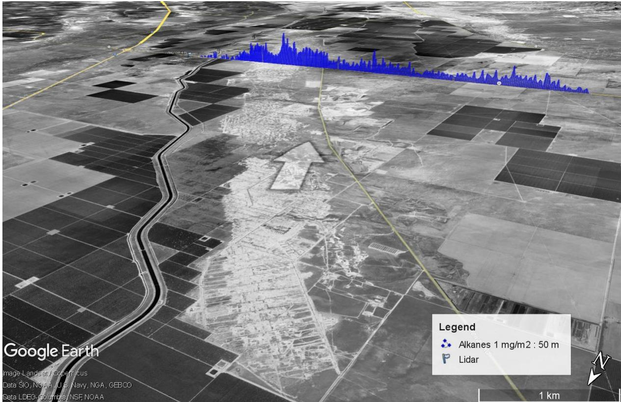
Figure 26. Alkane emission measurement of the north portion of the Lost Hills oil field 10 October 2021 , 12:50. The height of the blue contour corresponds to the measured column of alkanes where 50 m equals 1 mg/m<sup>2</sup>. The white arrow indicates the average wind direction during the measurement. Map from Google Earth™, 2021.
