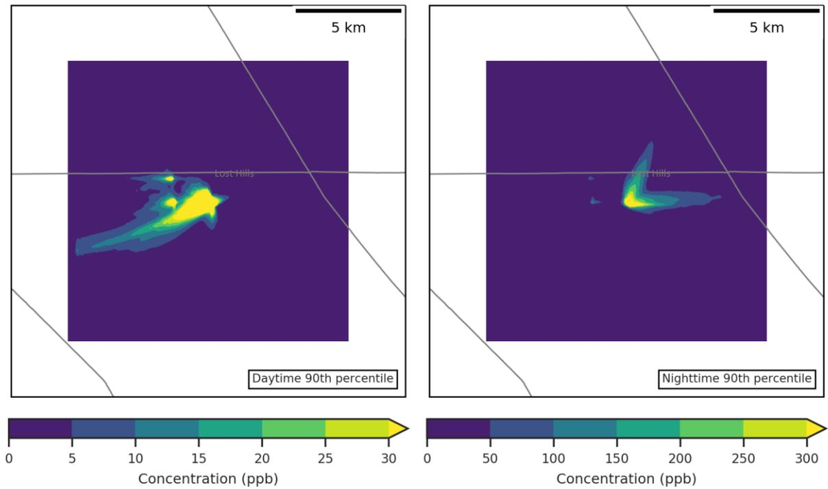
Figure 108 90<sup>th</sup> percentile of daytime (left panel) and nighttime (right panel) concentrations in the plume dispersion simulations for Lost Hills Processing 1 during the period 17-22 October 2021.
