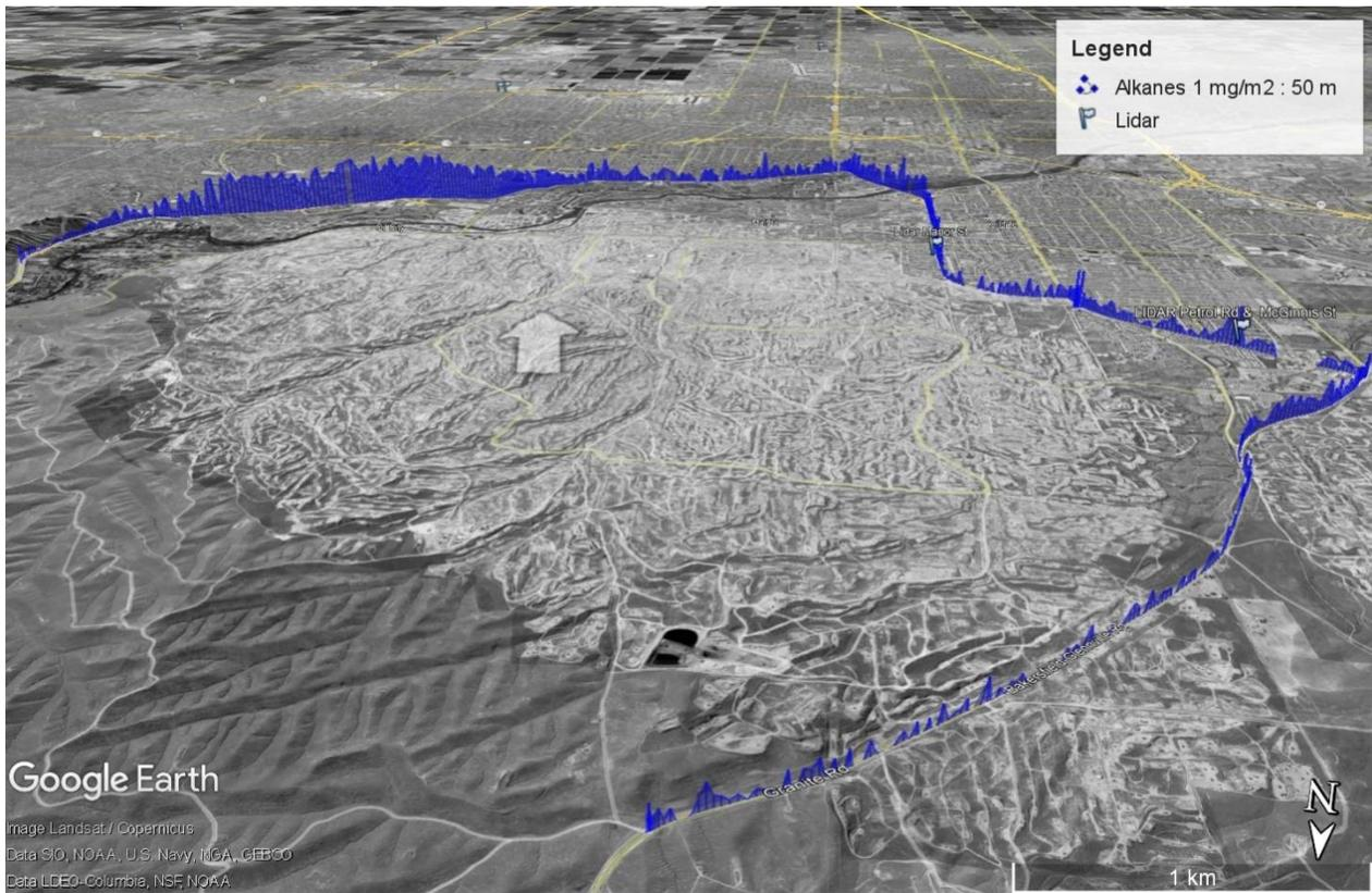
Figure 34. Alkane emission measurement by SOF of the Kern River oil field 16 October 2021 , 15:10. The height of the blue contour corresponds to the measured column of alkanes where 50 m equals 1 mg/m<sup>2</sup>. The white arrow indicates the average wind direction during the measurement (e.g. northerly wind here). Map from Google Earth™, 2021.
