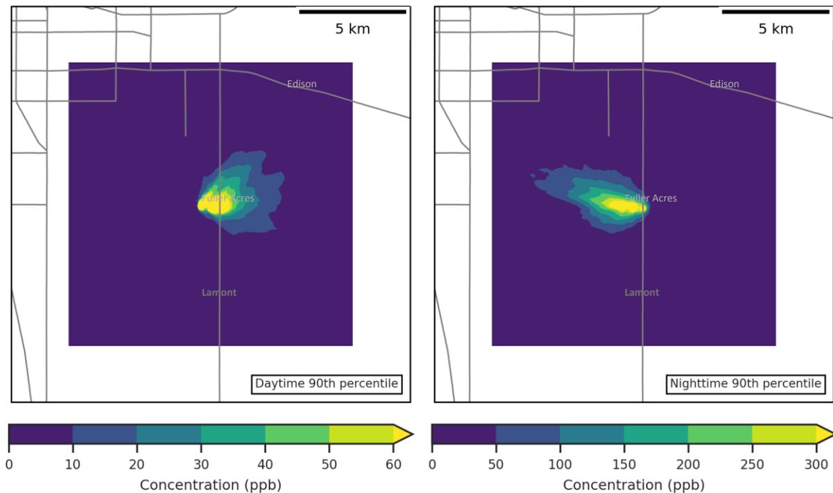
Figure 103 90<sup>th</sup> percentile of daytime (left panel) and nighttime (right panel) concentrations in the plume dispersion simulations for Kern Oil refinery during the periods October 12-14 and October 19-21.
