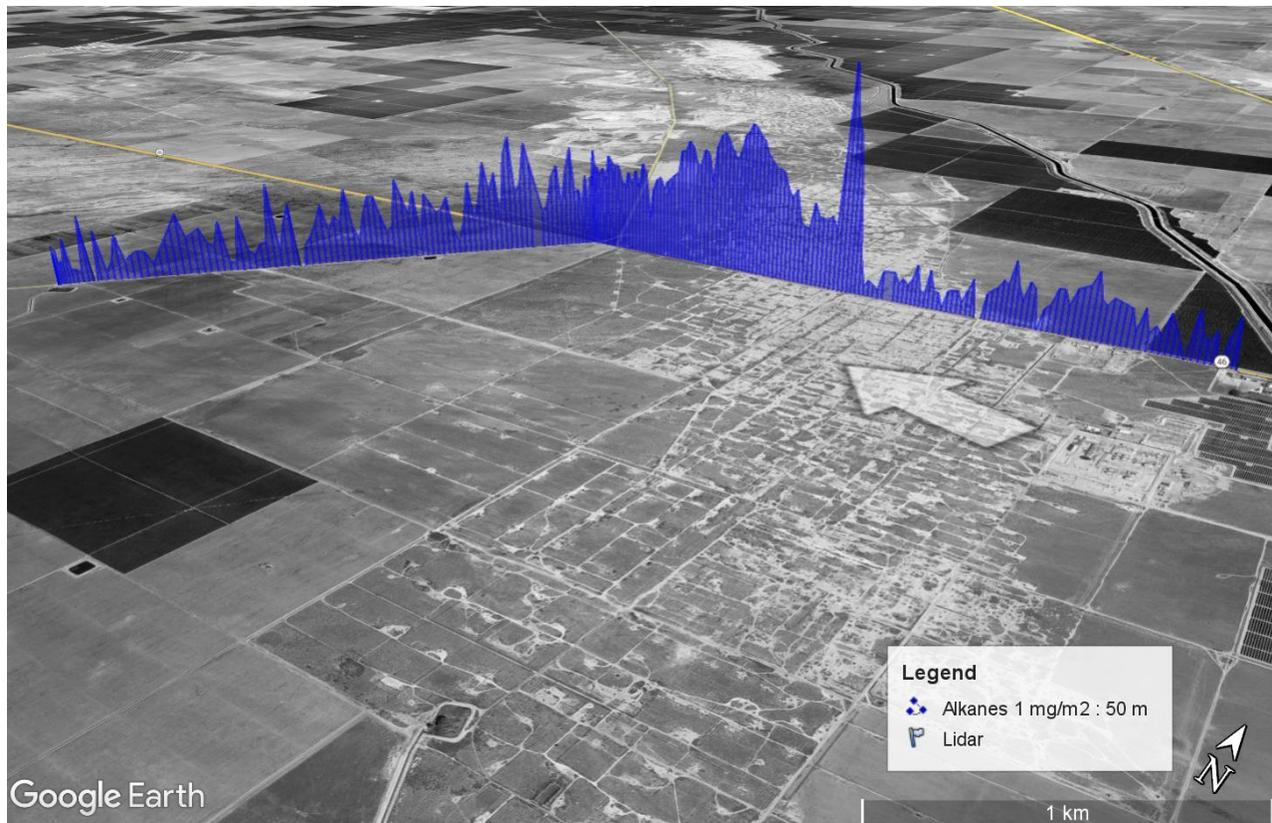
Figure 27. Alkane emission measurement of the Lost Hills south oil field 17 October 2021, 10:25. The height of the blue contour corresponds to the measured column of alkanes where 50 m equals 1 mg/m<sup>2</sup>. The white arrow indicates the average wind direction during the measurement. Map from Google Earth™, 2021.
