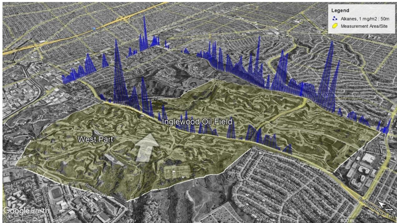
Figure 36. Typical SOF Alkanes measurement of the Inglewood oil field (Total and West Part) site 1 July 2021 at 12:00-12:30. The height of the blue contour corresponds to the measured column of alkanes where 50 m equals 1 mg/m<sup>2</sup>. The white arrow indicates the average wind direction during the measurement. Map from Google Earth™, 2021.
