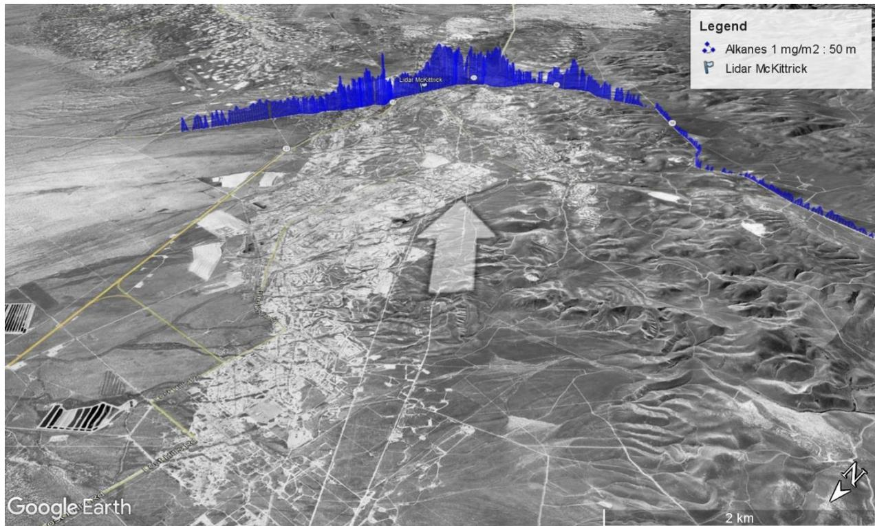
Figure 30. Alkane emission measurement of the Cymric & McKittrick combined oil fields on 11 October 2021 12:05. The height of the blue contour corresponds to the measured column of alkanes where 50 m equals 1 mg/m<sup>2</sup>. The white arrow indicates the average wind direction during the measurement. Map from Google Earth™, 2021.
