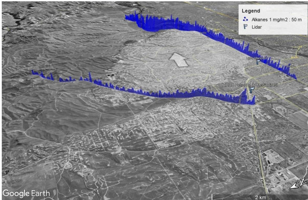
Figure 33. Alkane emission measurement of the Kern Front field (foreground) and the combined Kern Front + Kern River field emission plume (back end) on 15 October 2021, 13-14. Wind was blowing from west-northwest as indicated by the enclosed white arrow. The blue curve marks measured alkane column, where the height is scaled with the column having 1 mg/m<sup>2</sup> correspond to 50 m height above ground. Map from Google Earth™, 2021.
