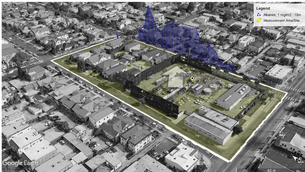
Figure 41. Typical SOF Alkanes measurement of the La Cienegas - Jefferson site 2 July 2021 at 16:10. The height of the blue contour corresponds to the measured column of alkanes where 10 m equals 1 mg/m<sup>2</sup>. The white arrow indicates the average wind direction during the measurement. Map from Google Earth™, 2021.
