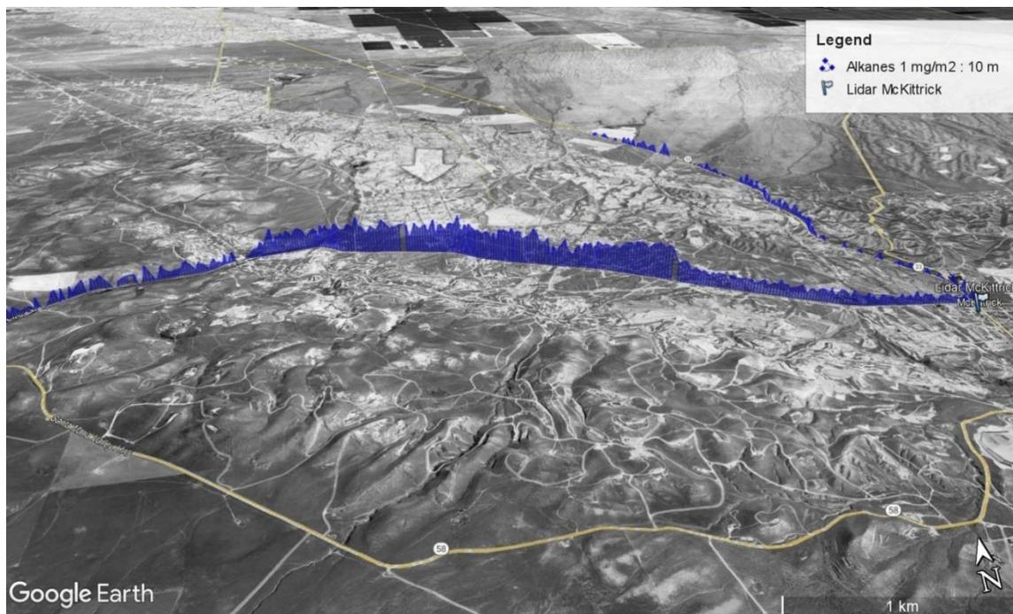
Figure 28. Alkane emission measurement of the Cymric field on 30 September 2021, 14:20. Wind was blowing from north as indicated by the enclosed white arrow. The blue curve marks measured alkane column, where the height is scaled with the column having 1 mg/m<sup>2</sup> correspond to 10 m height above ground. Map from Google Earth™, 2021.
