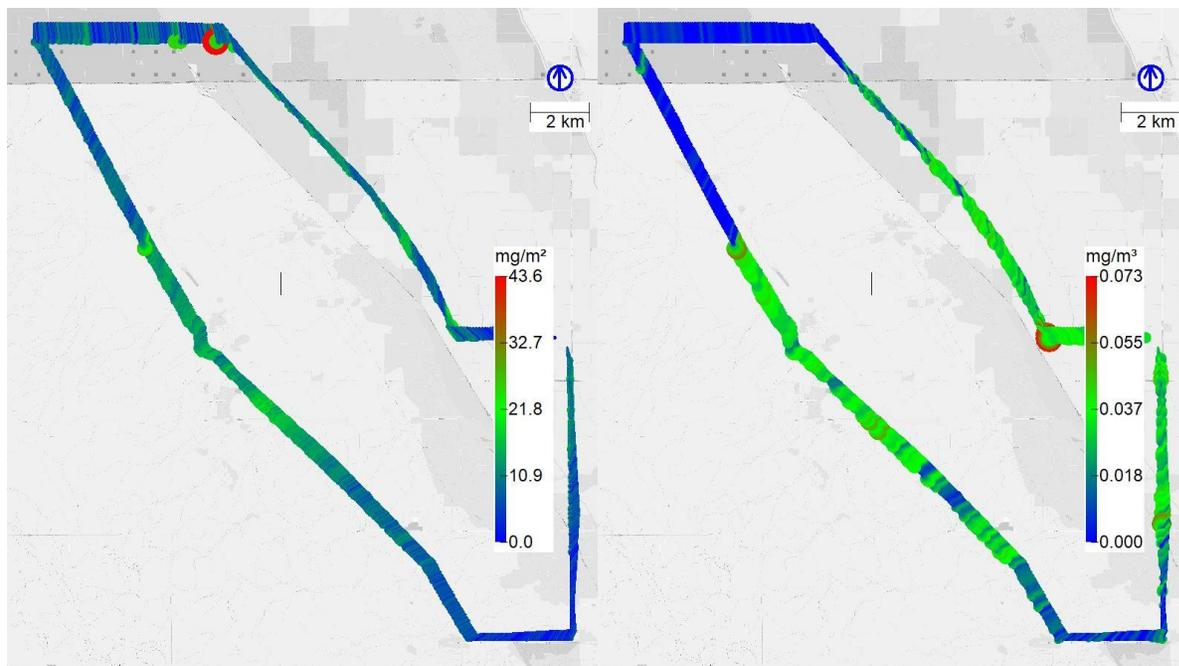
Figure 111. Plume height measurement example showing SOF alkane slant column (left) and MeFTIR alkane concentration (right) around Lost Hills. Two measurements are shown, one in the near field on Holloway and Highway 46 and the other in the far-field along Highway 33. The first order plume height estimates are 130 and 210 m, respectively.
