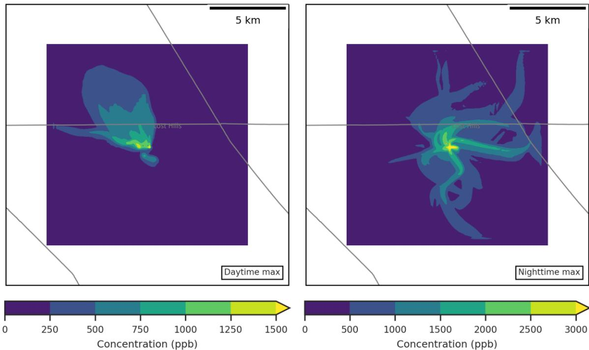
Figure 106 Maximum daytime (left panel) and nighttime (right panel) concentrations in the plume dispersion simulations for Lost Hills Processing 1 during the period 17-22 October 2021.
