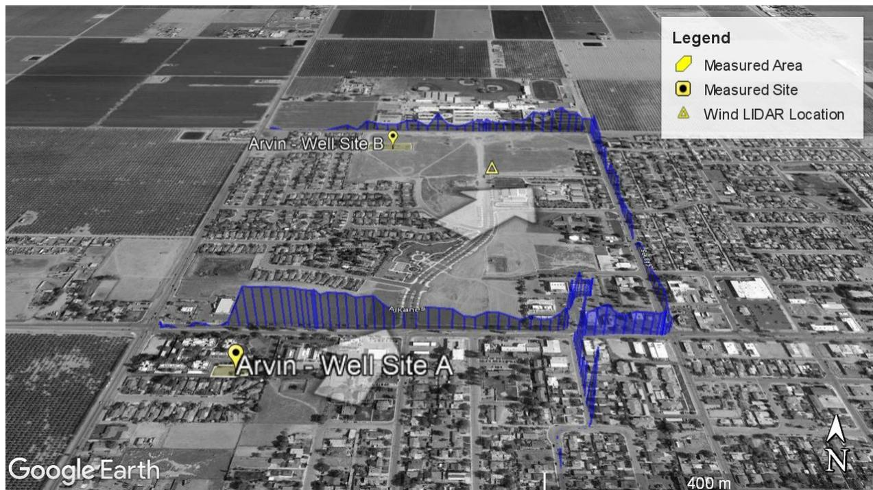
Figure 40. Two alkane emission measurements by SOF of the Mountain View Arvin well sites on October 12 2021, 15:00. Note there are other active wells and many plugged wells in this area not indicated on the image. The height of the blue contour corresponds to the measured column of alkanes where 10 m equals 1 mg/m<sup>2</sup>. The white arrows indicate the average wind direction during the measurements. Map from Google Earth™, 2021.
