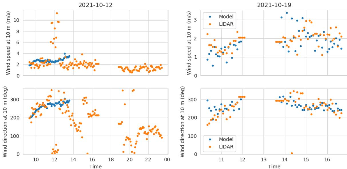
Figure 94 Comparisons of 10 m wind data as measured by wind LIDAR and as resulting from the WRF simulations for the Kern Oil refinery (at the location of the LIDAR). Data for October 12 is shown on the left and data for October 19 is shown on the right. The wind LIDAR was being moved (out of the model domain) around 12 o'clock on October 12, which explains the large deviations around that time.
