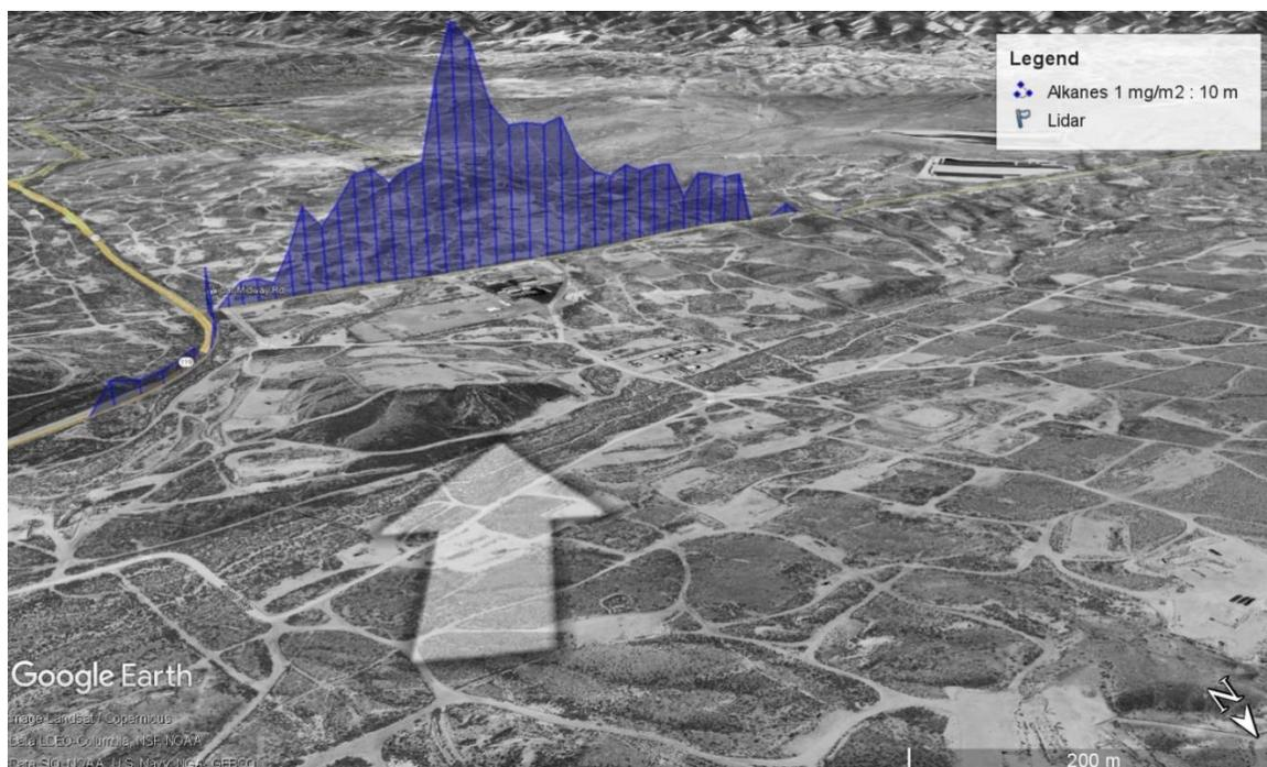
Figure 39. Alkane emission measurement by SOF of the Buena Vista Processing Site on October 14 2021 , 11:55. The height of the blue contour corresponds to the measured column of alkanes where 10 m equals 1 mg/m<sup>2</sup>. The white arrow indicates the average wind direction during the measurement (e.g. north-east here). Map from Google Earth™, 2021.
