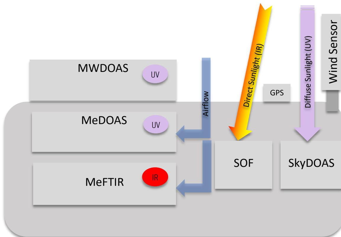
Figure 3. Overview of the mobile lab main instruments ; SOF, MeFTIR, MeDOAS (or MWDOAS) and SkyDOAS. SOF and SkyDOAS are column integrating passive techniques using the sun as the light source while MeFTIR and MeDOAS (or MWDOAS) measure near ground-level concentrations using active internal light sources.
