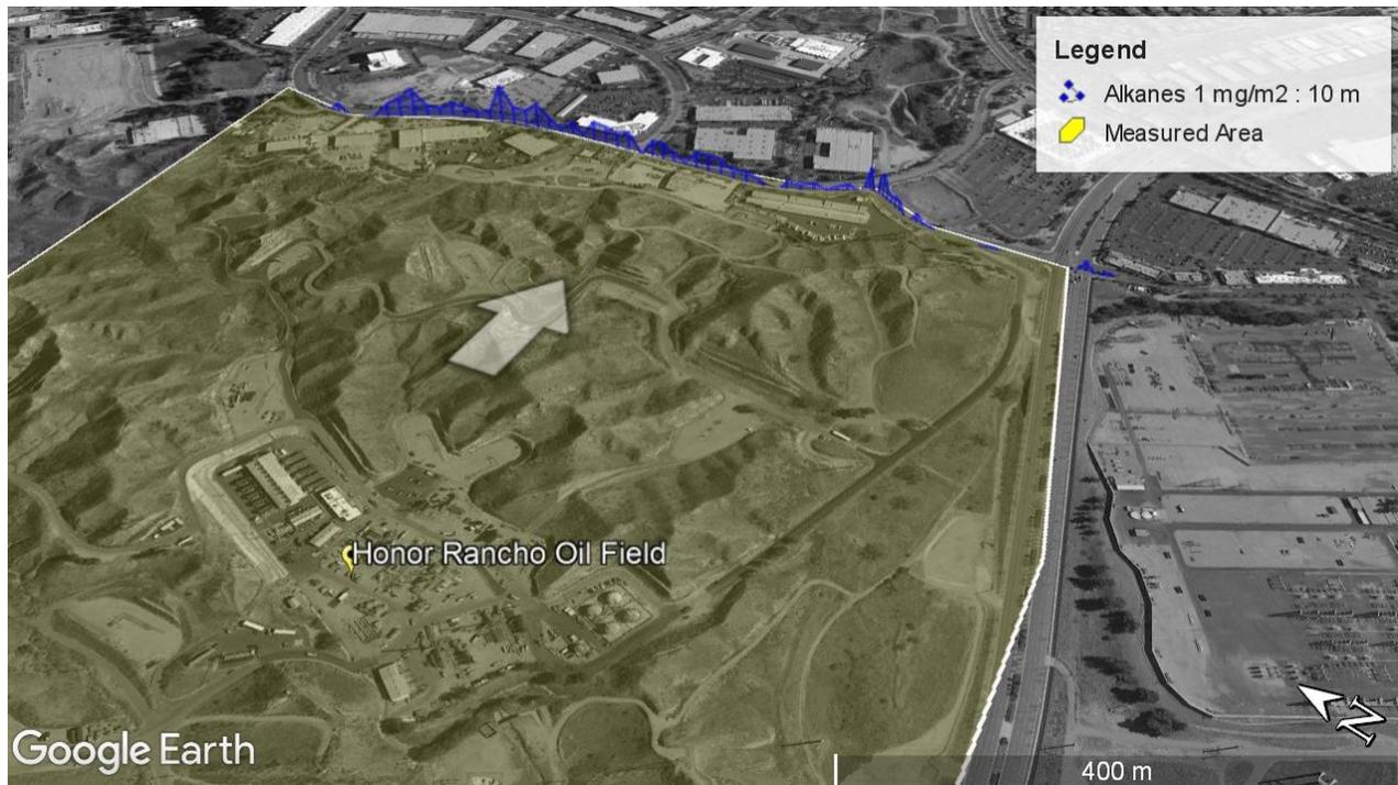
Figure 44 Example SOF Alkane measurement of Honor Rancho Oil Field 3 July 2021 at 11:13. The height of the blue contour corresponds to the measured column of alkanes where 10 m is equivalent to 1 mg/m<sup>2</sup>. The white arrow indicates the average wind direction during the measurement. Map from Google Earth™, 2021.
