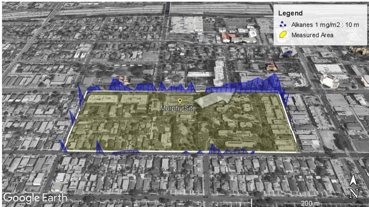
Figure 42 SOF Alkane measurement of the La Cienegas - Murphy site 25 June 2021 at 11:36 showing complete box measurement. Emissions were near the detection limit as seen in the upwind measurement here (to the southwest of the area). The height of the blue contour corresponds to the measured column of alkanes where 10 m is equivalent to 1 mg/m<sup>2</sup>. The white arrow indicates the average wind direction during the measurement. Map from Google Earth™, 2021.
