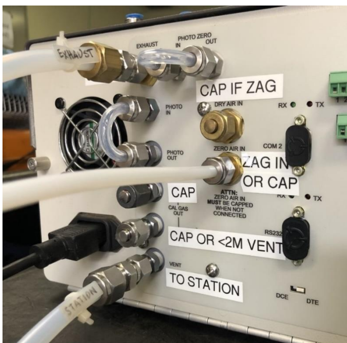
Figure C-2: Example tubing configuration for presentation through-the-probe using a length of 3/8" outside diameter tubing
