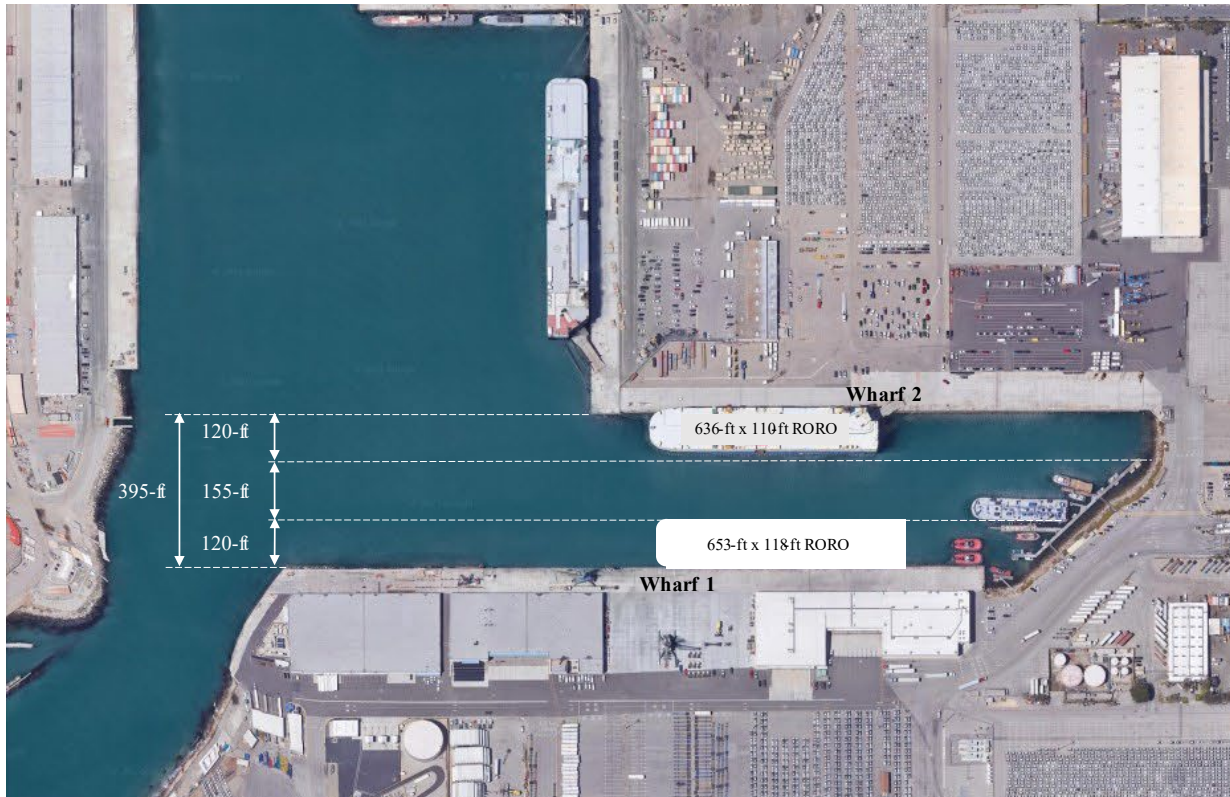
Figure 2-1: Channel width constraint when vessels are simultaneously berthed at Wharfs 1 and 2
