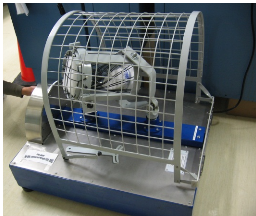
Figure 10. Three-dimensional Mixer - 88 Mixer System Schatz Model 4 (1A)
