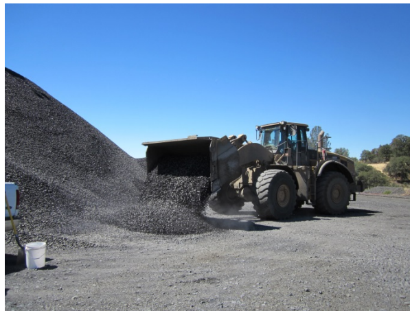
Figure 2B. Front Loader Sampling Aggregate Pile
