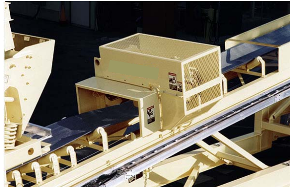
Figure 3B. Example of Automatic Conveyor Belt Sampler
