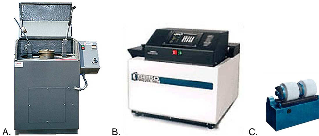
Figure 7. A. Vibrating Pulverizer (Shatter Box); B. Freezer Mill; C. Ball Mill
