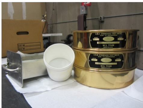
Figure 13. Stack of Sieves for Particle Size Check
