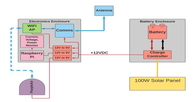
Power will be generated using solar panels and a solar charge controller in conjunction with a single battery. The battery will be housed in an enclosure separate from the electronics. Communications will be achieved through the use of a satellite terminal or cellular modem.
