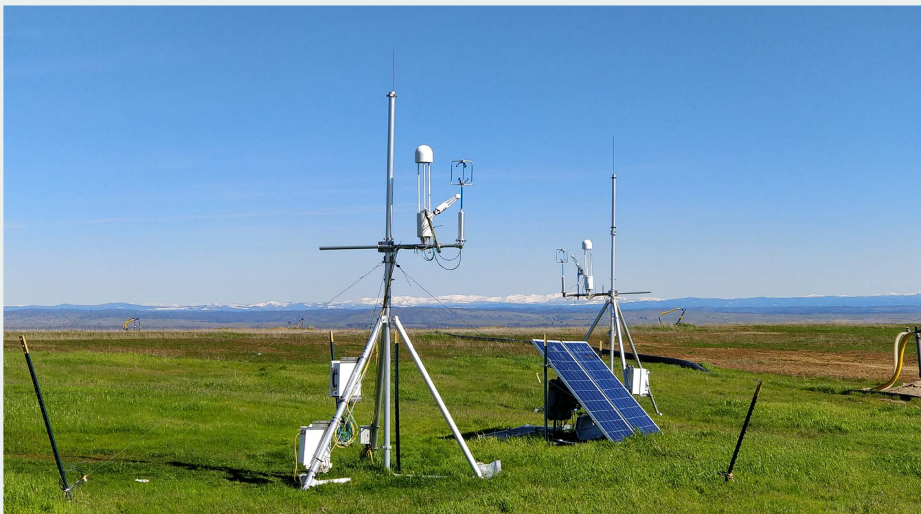
Figure 28: Flux tower deployed in the field
