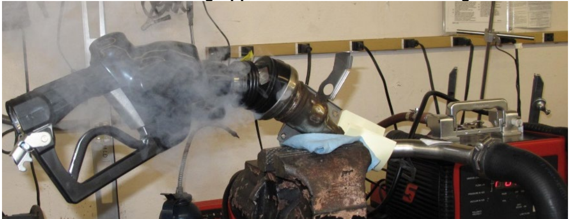
Figure V-6 Smoke Testing Apparatus Used for Leak Testing
