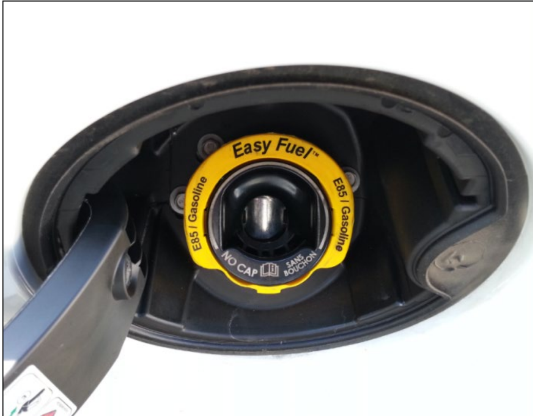
Figure V-3 Capless Fill Pipe System
