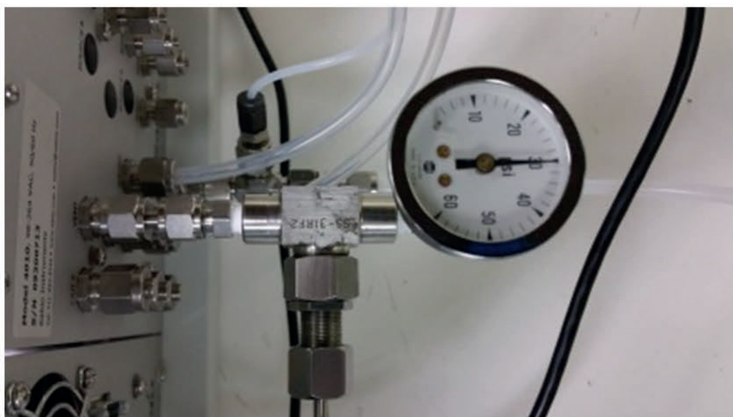
Figure 19: T-valve and Pressure Gauge Connection.
