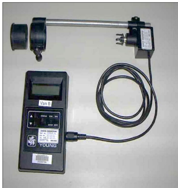
Figure S.11 R.M. Young Anemometer Drive with Motor Assembly
