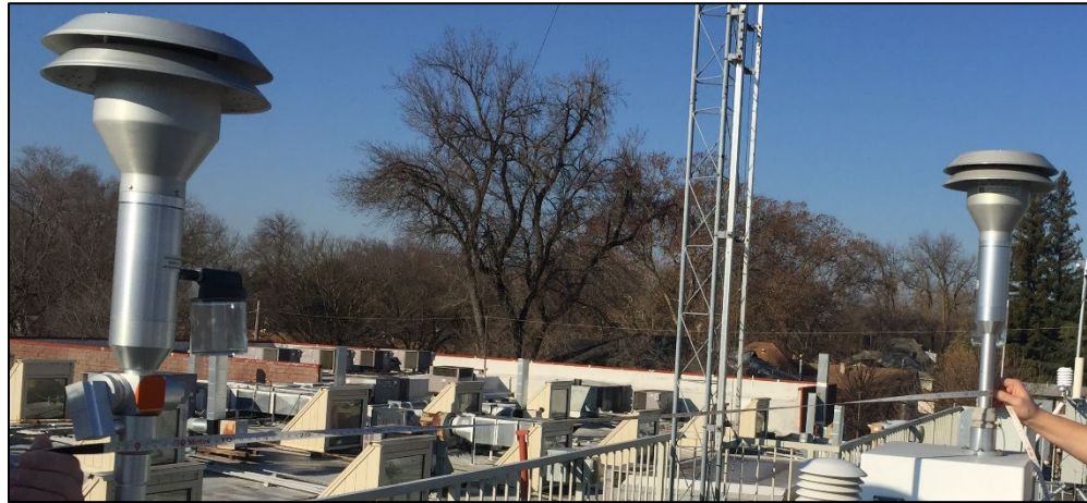
Figure AE.12 Measuring Distance between Inlets of Two Samplers
