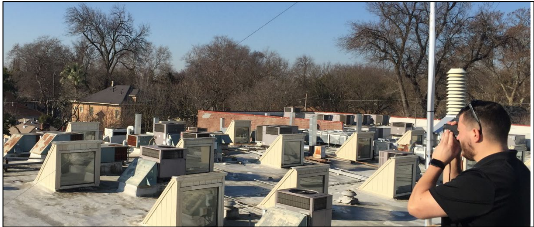
Figure AE.14 Utilizing a Rangefinder to Measure Inaccessible Obstacles
