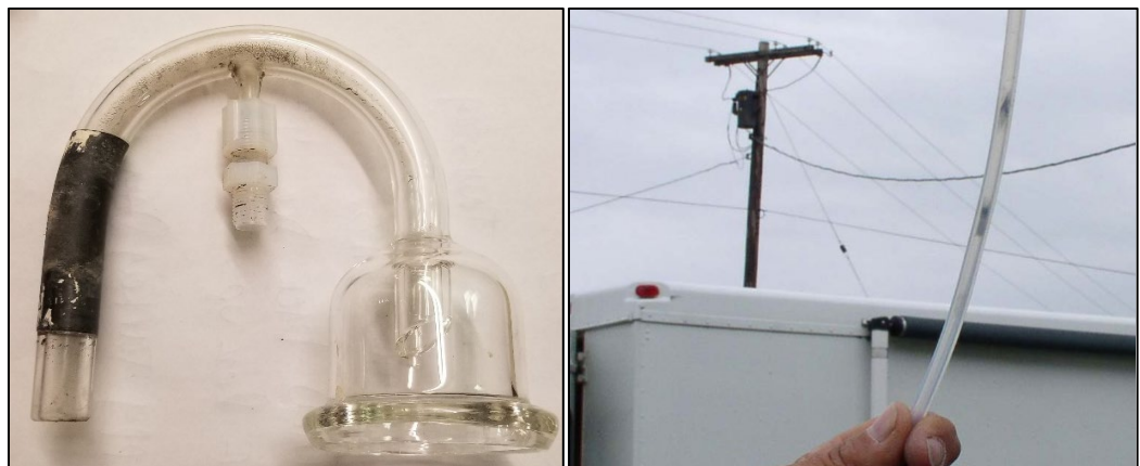
Figure AE.16 An Example of a Dirty Probe and a Sample Line with Spider Webs
