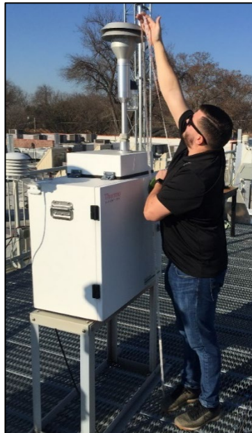
Figure AE.13 Measurement of Inlet Height above Roof or Platform
