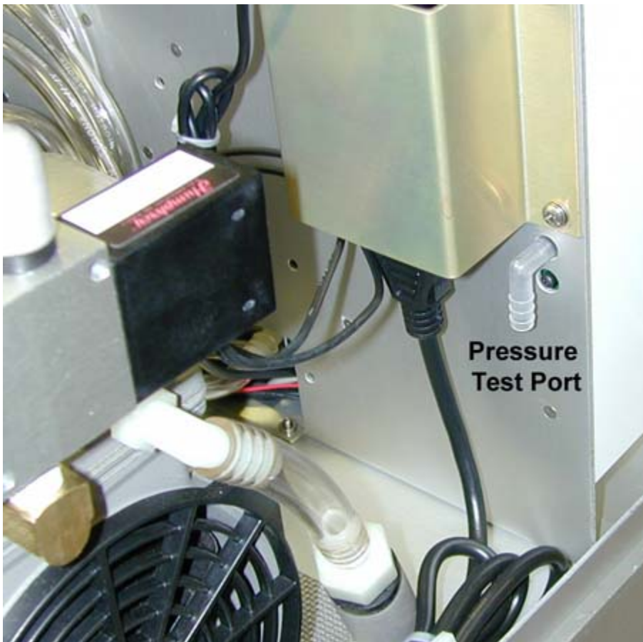
Figure 5: Pressure Test Port Location
