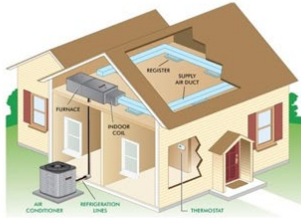
split systems (ducted)
