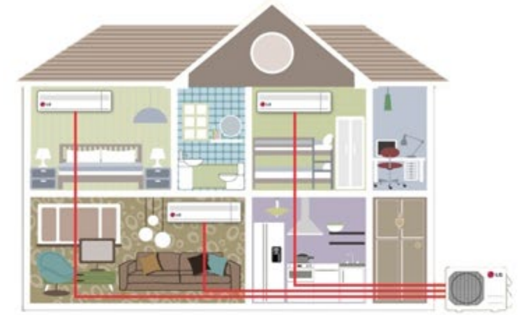
split systems (ductless)
