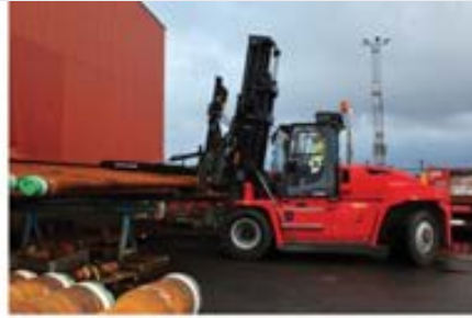
Two (2) 21-ton electric forklifts
