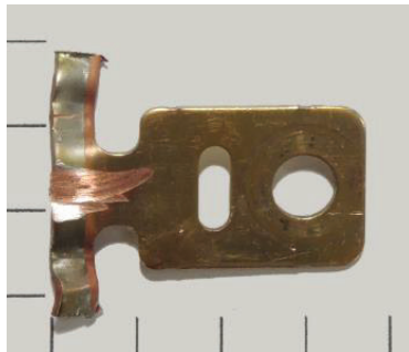
Figure D-8 Chevy Volt Stator Spade Terminal
