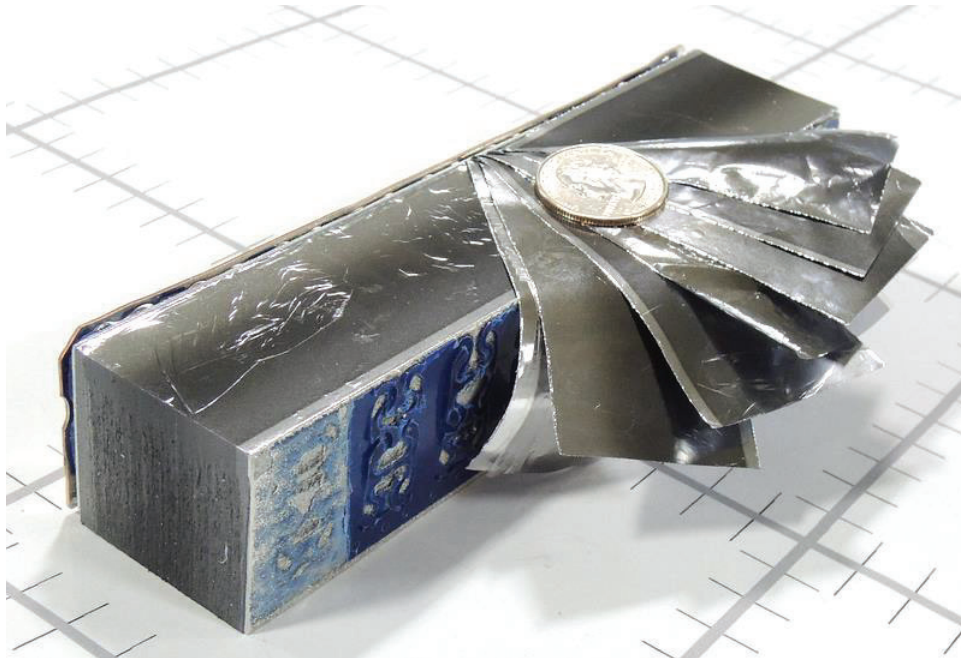
Figure F-45 Audi Inverter: Capacitor Film Assembly Showing Metallized PP Film
