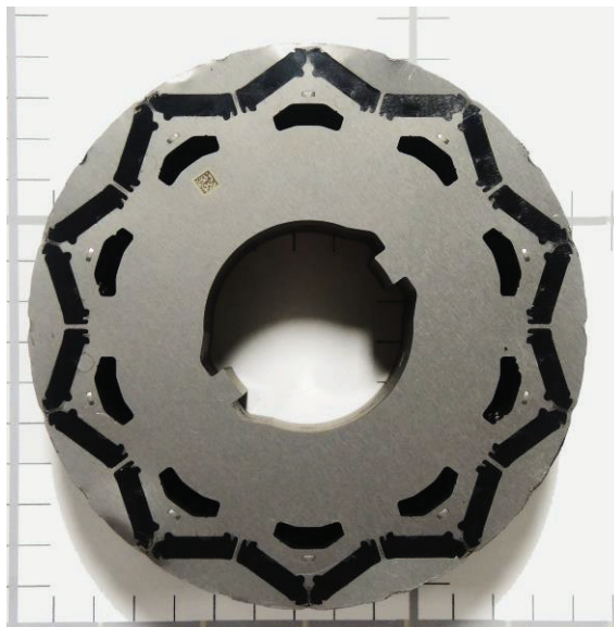
Figure B-13 Toyota Prius Rotor 10-Pole Magnet Configuration
