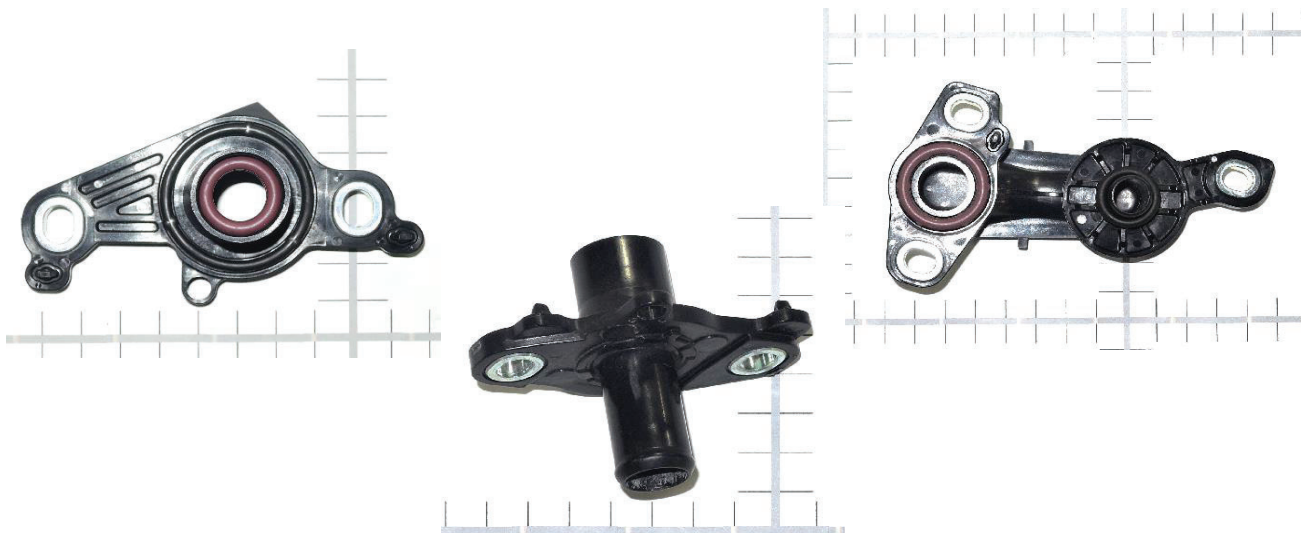
Figure C-10 Toyota Coolant Fittings: IGBT Cooler Interface (Top Left), DC/DC Cooling Interface (Top Right), IGBT to Vehicle Outlet Adapter (Bottom)
