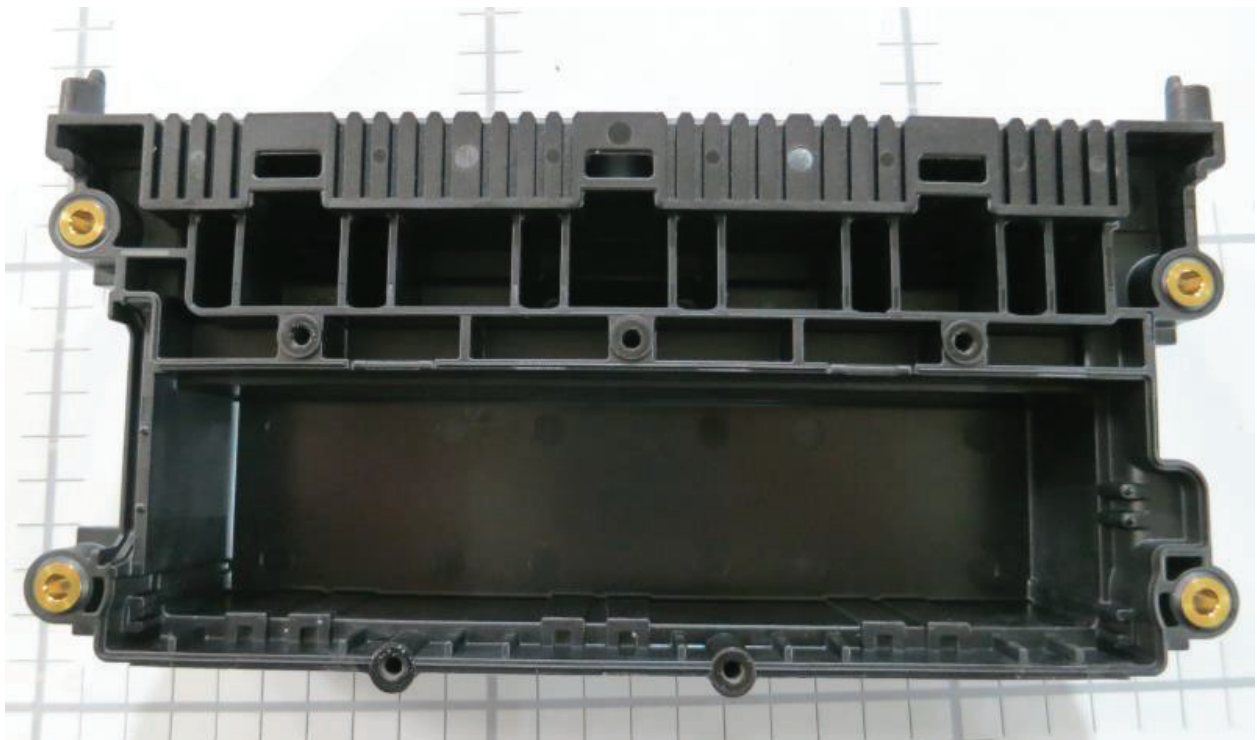
Figure F-46 Audi Inverter: Capacitor Housing
