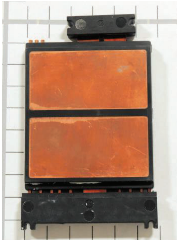
Figure F-42 Audi Inverter: IGBT Half Bridge Assembly (Top), IGBT with Connectors and Terminals (Bottom)
