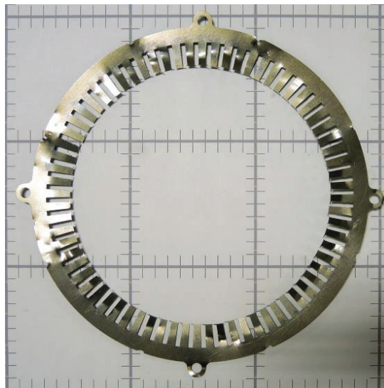
Figure D-3 The Chevy Volt Stator Laminate Segment
