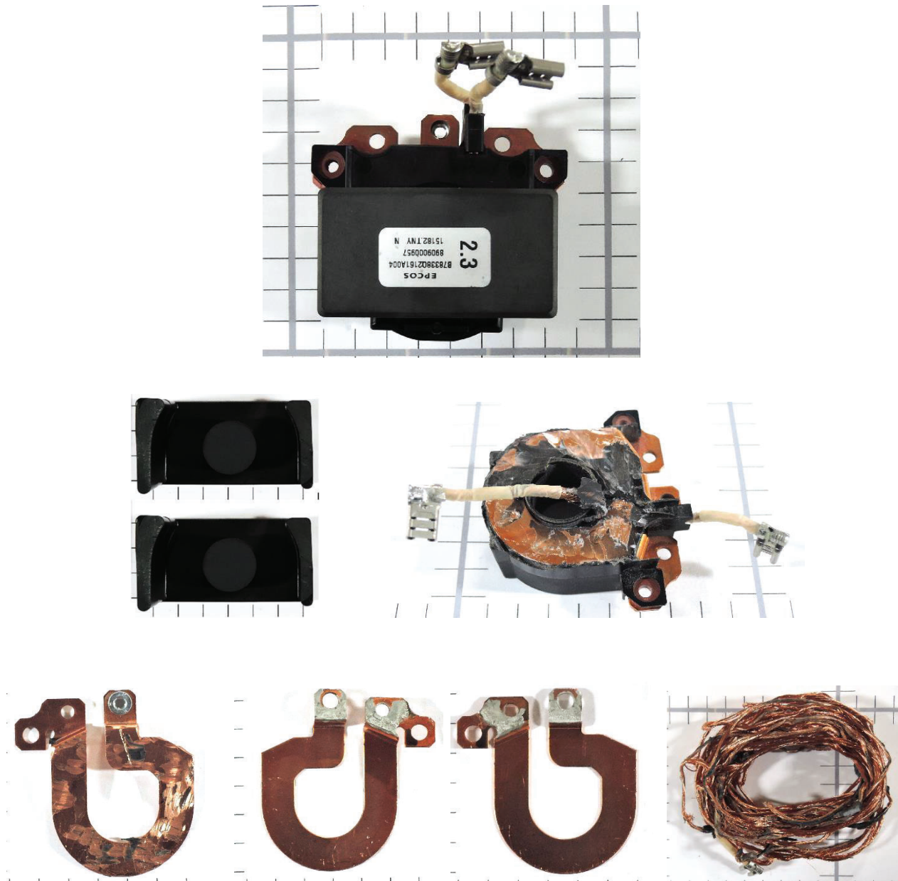
Figure F-29 Audi DC/DC Converter: Assembled Transformer top, Ferrites Center right, Inductor Assembly minus Ferrites Center left, bottom: Stamped Copper Plates left, Copper Wire right
