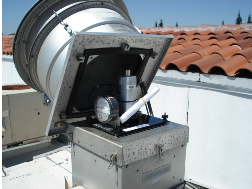
Figure 6: Installed BGI Variable Orifice
