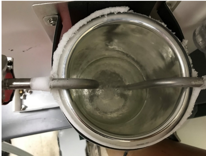
Figure 5. U-trap Inside Liquid Nitrogen Dewar
