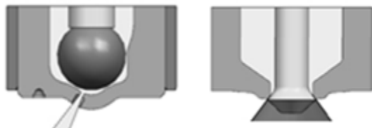
Figure 5 - Inwardly and outwardly opening injector tips - Delphi-Piock-eng 2015 Vienna
