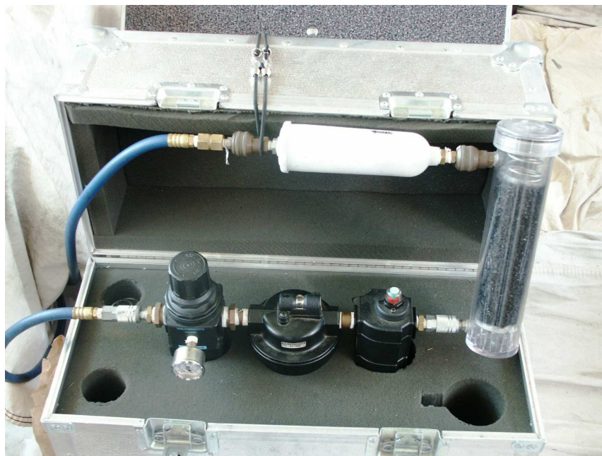
Figure A- 2 Field Processing Unit for Purifying Dilution Air in Transport Case
