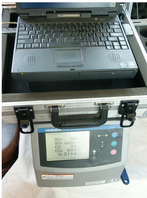
Figure A- 3 In-field Illustration of Continuous Gas Analyzer and Computer for Data Logging
