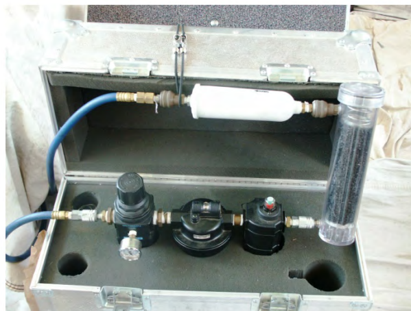
Figure B-2: Field Processing Unit for Purifying Dilution Air in Carrying Case
