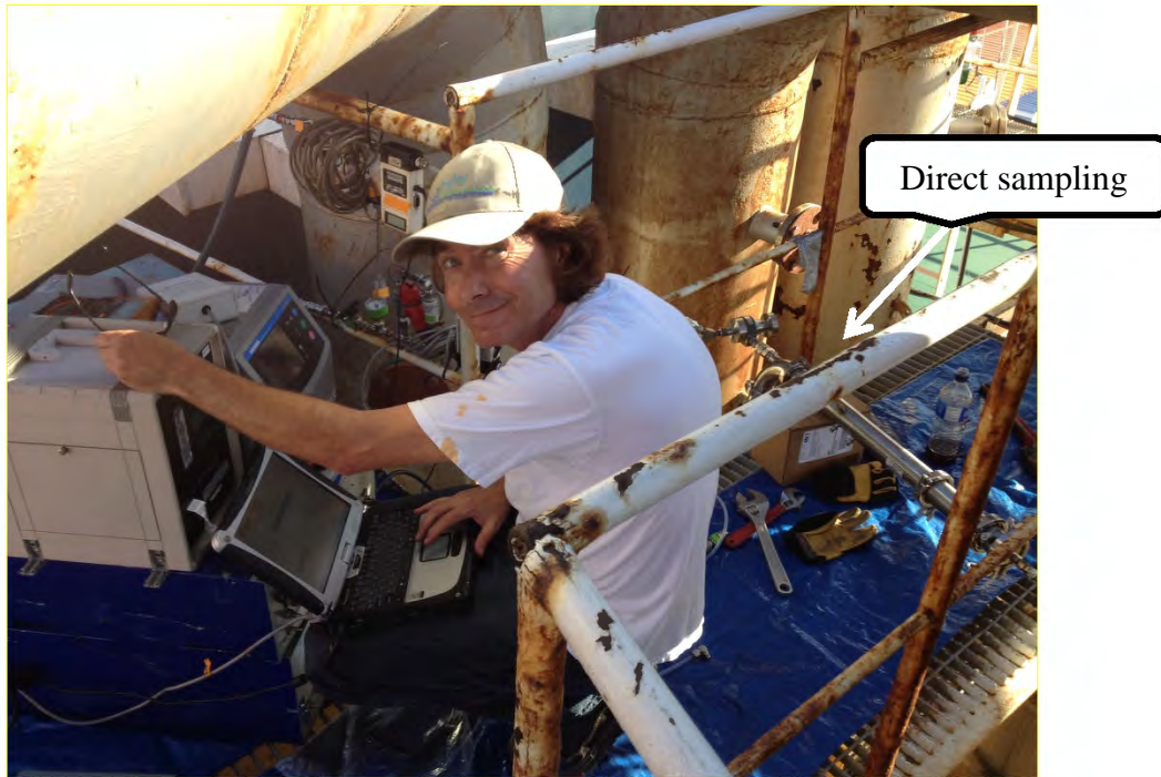
Figure C-2 Dilution system and measurement layout on the auxiliary engine exhaust stack
