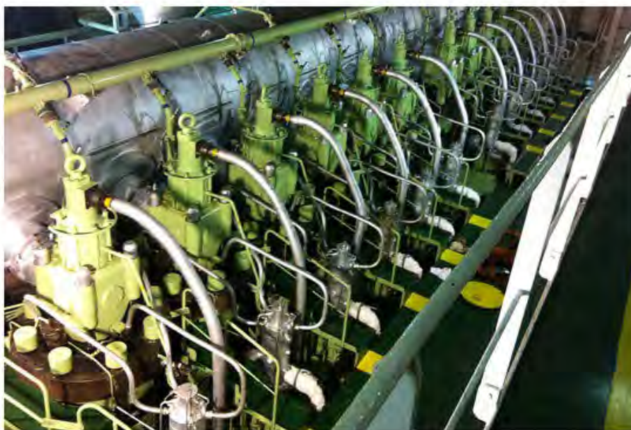
Figure 3-1 Samsung-MAN B&W main propulsion engine tested under voyage
