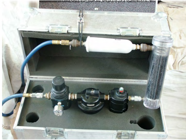
Figure C-3 Field Processing Unit for Purifying Dilution Air in Carrying Case
