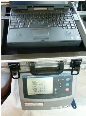
Figure C-4 Setup Showing Gas Analyzer with Computer for Continuous Data Logging
