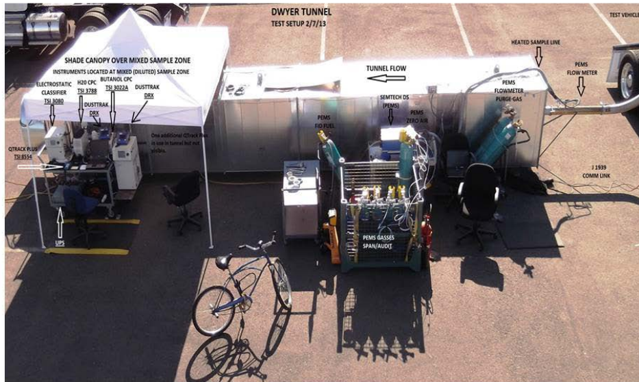
Figure II-5 Photograph of small wind tunnel and emission instrumentation
