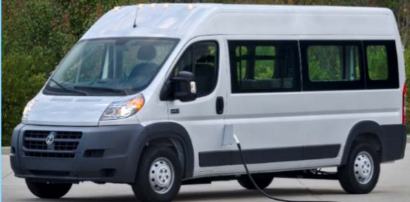
Cargo/Passenger Van Shuttle and local operations 50-100 miles per charge 30-60 kWh battery
