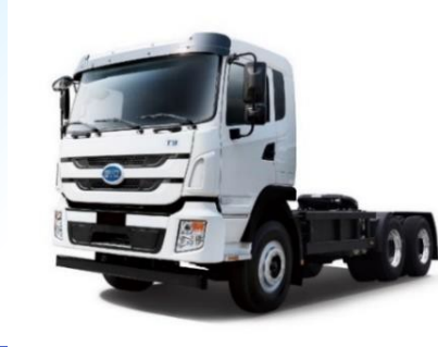
Drayage Truck Port goods movement 100 miles per charge 188 kWh battery
