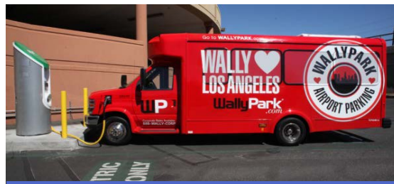
Cutaway Bus Airport and transit shuttle 100 miles per charge 105 kWh battery
