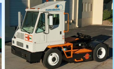
Yard Tractors Intermodal operations ~60-80 miles per charge ~209 kWh battery
