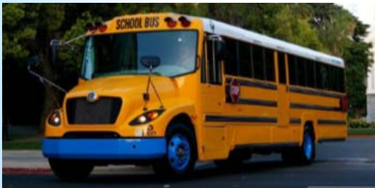
School Bus Type A, C, and D operation 50-150 miles per charge 65-200 kWh battery
